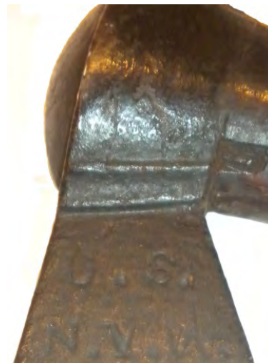
Figure 30. Type III boarding axe reinforced socket bowl; note the reinforcement between the blade and socket.
