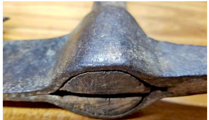
Figure 22. Type I Axe rivet perpendicular to wedge.
