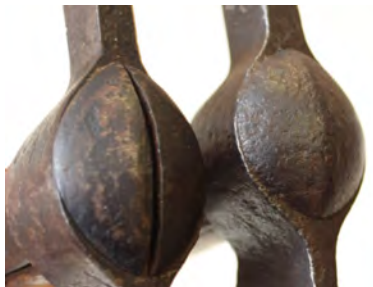
Figure 28. Side by side split (left) and solid cap (right) Type III boarding axes.
