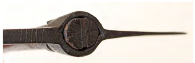
Figure 23. Type I axe rivet through wedge.
