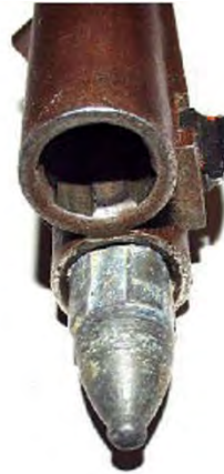
Figure 3. Muzzle of Jacob rifle showing four-land rifling and matching four-lug explosive projectile. ( www.gunrightsmedia.com , The Jacob Rifle)
