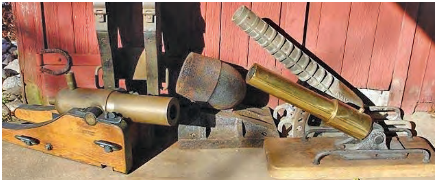
A Hall-Naval Company Model F cannon (right rear). Part of a great collection of line throwing artillery. Left to right Lyle Model C cannon for the U.S. Life Saving Service, a U.S. 24 Pounder Eprouvette “Manby mortar” and early Hunt line throwing cannon.
