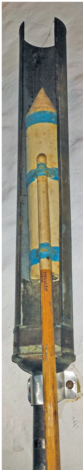
Trengrouse launcher attachment to adapt muskets for line throwing. Courtesy Helston Museum, Helston, Cornwall, UK
