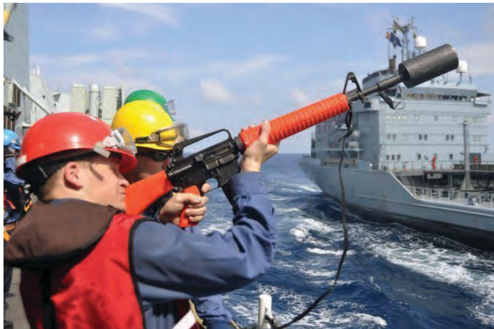
Canadian sailor using M16 (C7) rifle with Mark 87 line throwing adapter. Photo courtesy Canadian Maritime Forces Atlantic (MARLANT), CFB Halifax.
