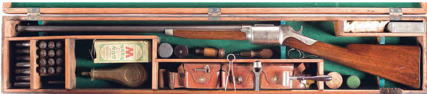
FIGURE 10: Cased Sylvester H. Roper revolving shotgun, U.S. patent from 1866, produced through 1876. It uses separate-primed, reloadable steel cartridges, seen muzzle-down and on their sides at the left. (Photo: Rock Island Auction)
