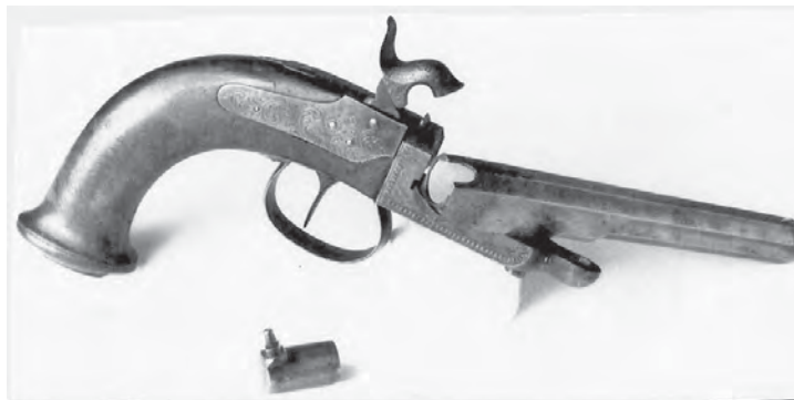
FIGURE 8: A reloadable cartridge with copper-cap nipple, constructed for an external hammer.
