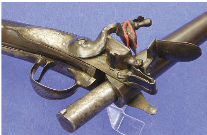
FIGURE 4: The Freeman gun's reloadable iron cartridge. The lug at the end allows alignment of the barrels and cartridge's touchholes. (Photo: Bolk Antiques)
