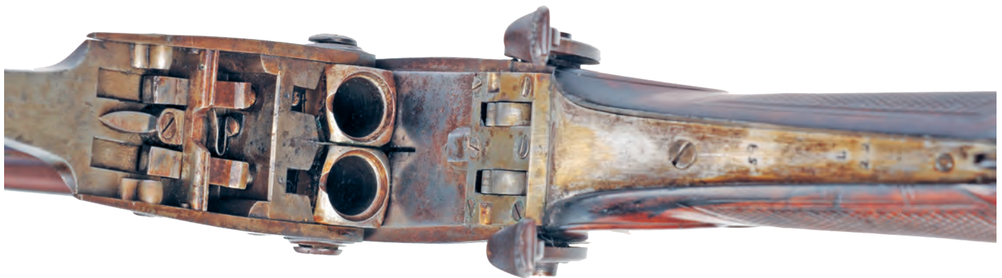
FIGURE 17: Inside the double gun action. RIGHT: Hammers (the protruding ends of the tumblers) cocked. MIDDLE: Breech openings for rimmed cartridges. LEFT: The bascule fully raised, with the spring-controlled firing pins. With the action closed, the firing pins will be within reach of the hammers. (Photo: Dan Retting)
