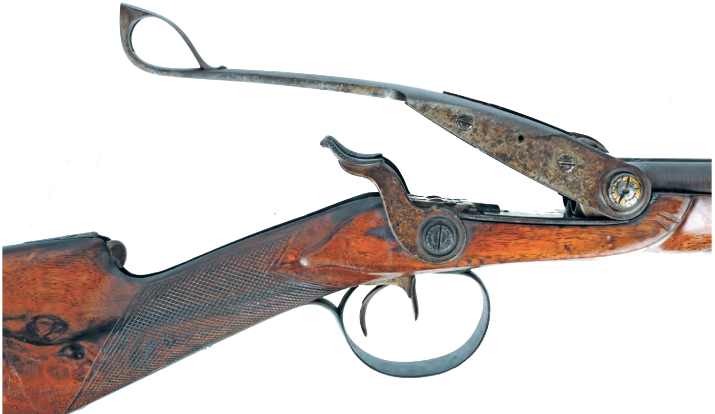
FIGURE 16: The "bascule" partly open. (Photo: Dan Retting)
