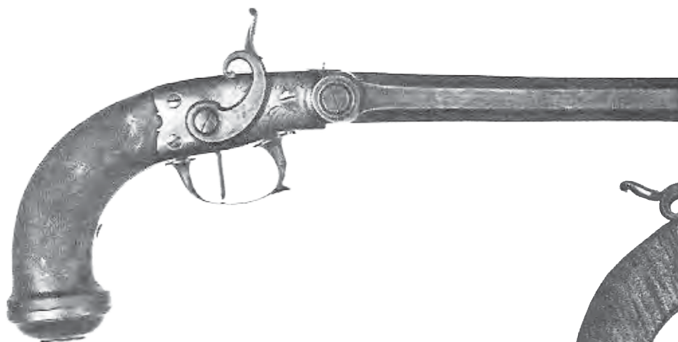
FIGURE 13: A Pauly pistol, closed. Note the external cocking lever. 5 Winant, p. 26.
