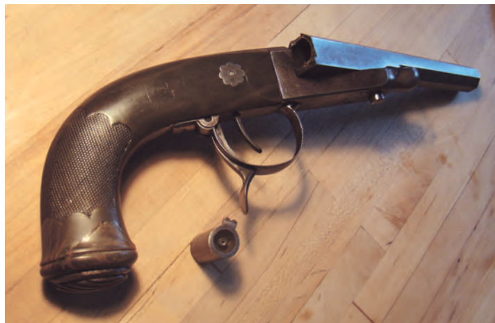
FIGURE 9: Another cartridge with copper-cap nipple, constructed in-line for an internal striker. Note the unusual design choice, placing a rear sight on each cartridge. (Photo: Peter Bower)
