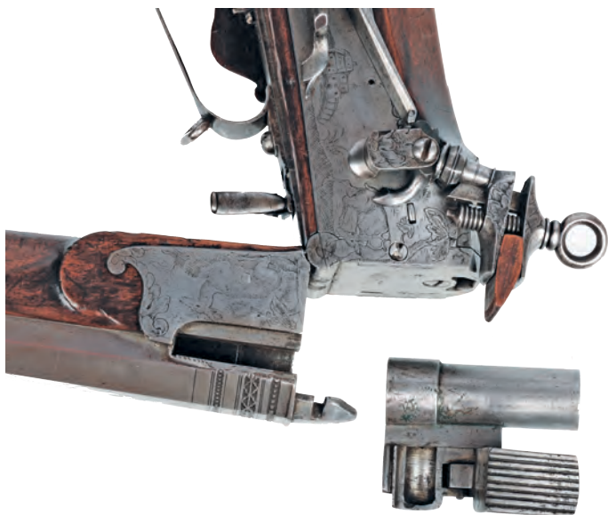
FIGURE 7: A reloadable cartridge with integral pan and frizzen. (Vienna, circa 1650.) (Photo: Dan Retting)
