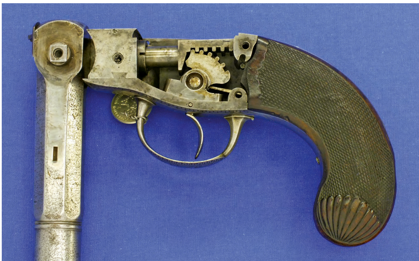
FIGURE 29: Pauly fire-piston pistol action, cocked. Note the piston plunger, and gearing. (Photo: Bolk Antiques)
