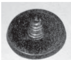
FIGURE 20: Top: the inside of a paper cartridge rosette. The screw helps attach the rosette and cartridge. The ignition channel passes through the center of the screw.
