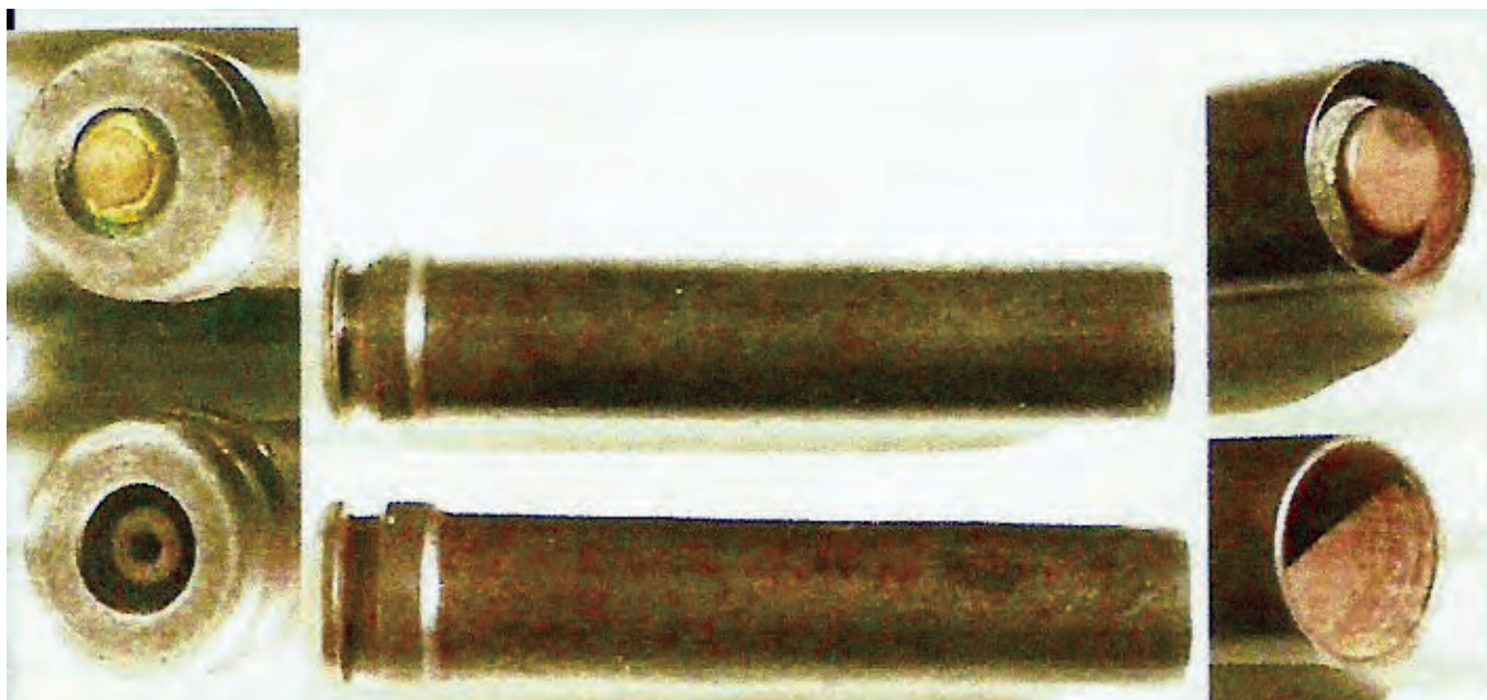
FIGURE 11: A group of Roper revolving shotgun and rifle cartridges. Lower left: earlier, with copper-cap-primed nipple. Top: later, using assorted primers pressed into the base. Bottom right: the open muzzle end, for loading. (Photos: Pete deCoux)
