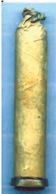
FIGURE 19: A Pauly gun paper cartridge, with the brass base ("rosette") seen from the side. (Photo: Jim Gooding)
