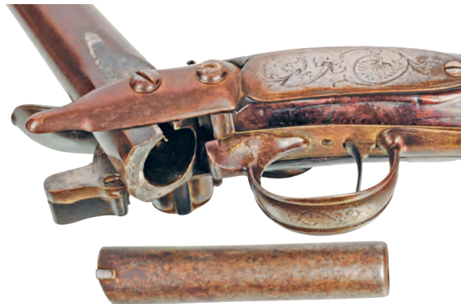
FIGURE 5: The Freeman gun's 4 1/2" cartridge fully removed. Note the breech open, with a cutout for the alignment lug. (Photo: Dan Retting)
