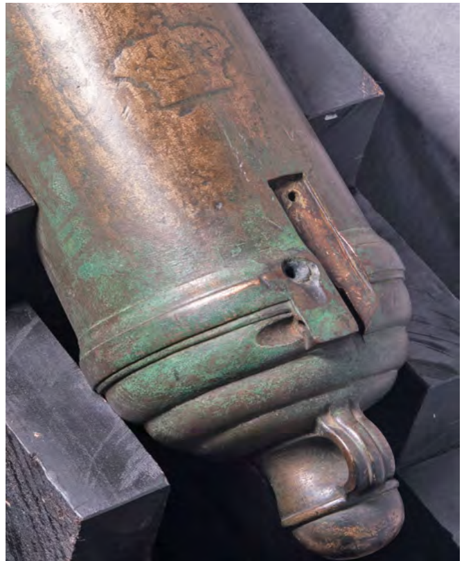
Figure 25. A ca. 1820 naval Carronade showing a mortise for mounting a cannon lock. Vallejo Gallery, Costa Mesa, California.
