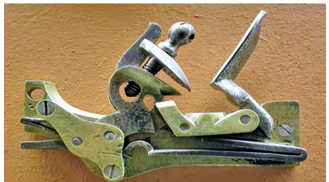
Figure 27. The inside of a late 1700s lock showing the sear and mainspring. Pitt Rivers Museum, University of Oxford, Oxford, England.
