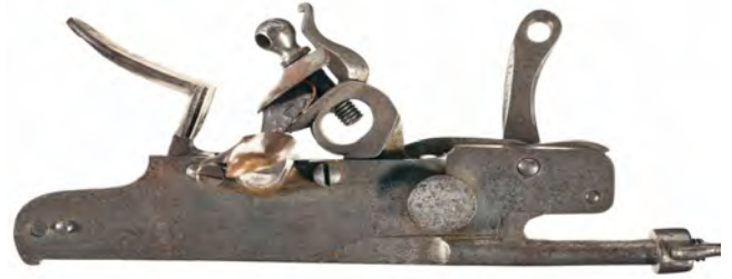
Figure 29. A French lock featuring a long tail bolt with a wing nut, extended pan cover and a tall lanyard pull lever. Vikingsword.com., Ethnographic Arms & Armor Forum.
