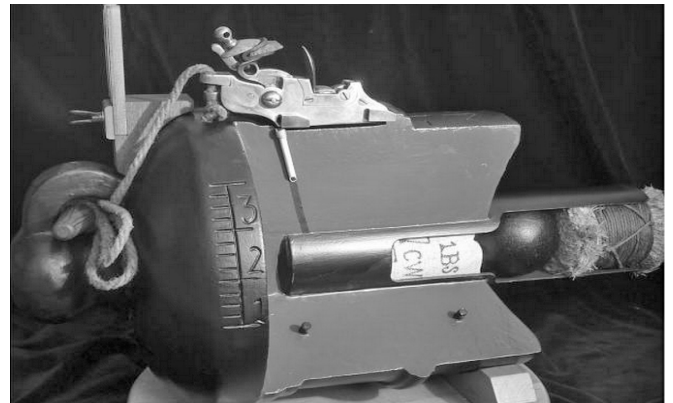
Figure 5. A cutaway view of a flintlock mounted on a Bloomfield cannon barrel, showing a quill or tin tube primer, the powder charge, round ball and wad. Thomas Bloomfield was Inspector of Artillery at Woolwich, England in 1780 and developed a new standardized system of gun design which was implemented in 1785. Note the long flame path from the lock to the charge. The pans of these flintlocks are significantly larger than conventional small arms locks, to ensure enough flash to reach the charge. Photo from Game-Labs forum.
