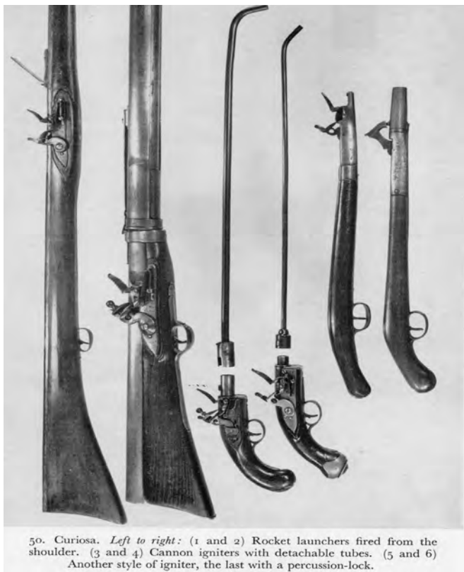
Figure 35. This is a page from Howard Blackmore's book " British Military Firearms 1650-1850 ". Entitled "Curiosa", it shows four ignitors. Two of these are flintlock pistols fitted with long extension tubes, one attached by a lug and the other by a threaded screw. 6
