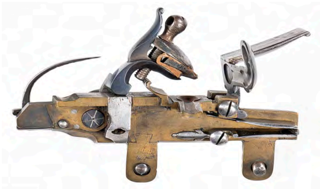
Figure 13. An unusual lever firing mechanism and extended mounting bars with pins. This lock also features an extended pan channel and cover mounted to the frizzen. Australian Arms Auctions.
