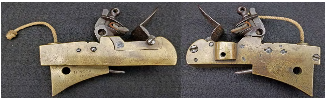
Figure 26. A Carronade lock made by H. Nock and dated 1801. Henry Nock (1741-1804) was an English gunmaker of great renown, becoming a Freeman of the Gunmakers Company in 1784 and was elevated to Master in 1802. Mike Edwards collection.
