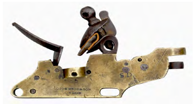
Figure 6. A typical British pattern lock by C. Johnson & Son, London. It is unconfirmed what the “SD” mark signifies. This lock features holes at its base for mounting horizontally to a cast platform at the cannon’s vent hole with the use of bolts. The cock is released by a lanyard attached to the bottom ring at the rear of the lock, which is then threaded up through the upper ring. Matt Sears collection.
