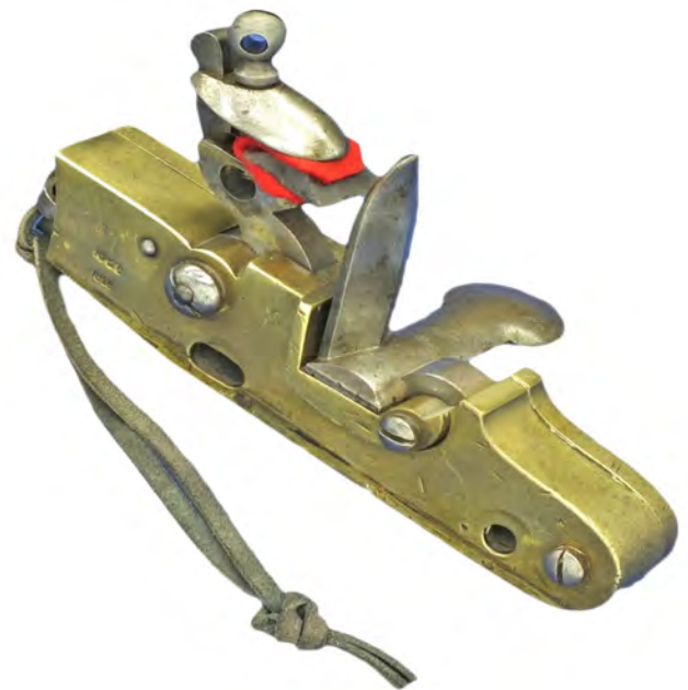
Figure 21. This lock is from Denmark and dates to 1828. It is marked crown over FR and KGE. Notice the extended pan cover attached to the frizzen, which has a circular form at its end to cover the cannon's vent hole. Matt Sears collection.
