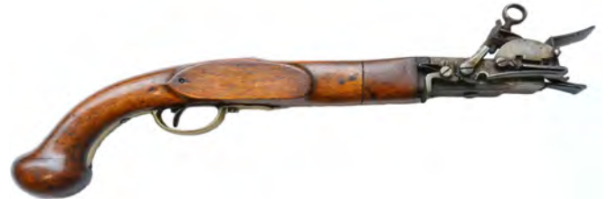
Figure 32. This early 1780s French hand-held flintlock ignitor functioned much like the slowmatch/portfire system. It features a belt clip, brass furniture and an enlarged pommel on the grip for wet weather use. Tennants Auctions, London, England.
