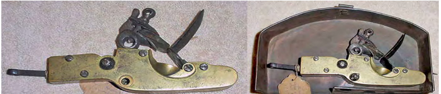
Figure 8. This lock by an unknown maker is also shown housed in its copper casing (right). The copper enclosure, as shown, is incomplete, missing a clip-on closure cover. It is assumed that the purpose was for weather protection to enable locks to remain fully charged while awaiting use. These were eventually abandoned due to ineffectiveness and added complexity. Notice that the mechanisms throughout this article vary with the method of connecting the lanyard to activate firing. This one uses a linear pull trigger. Dick Salzer Collection.
