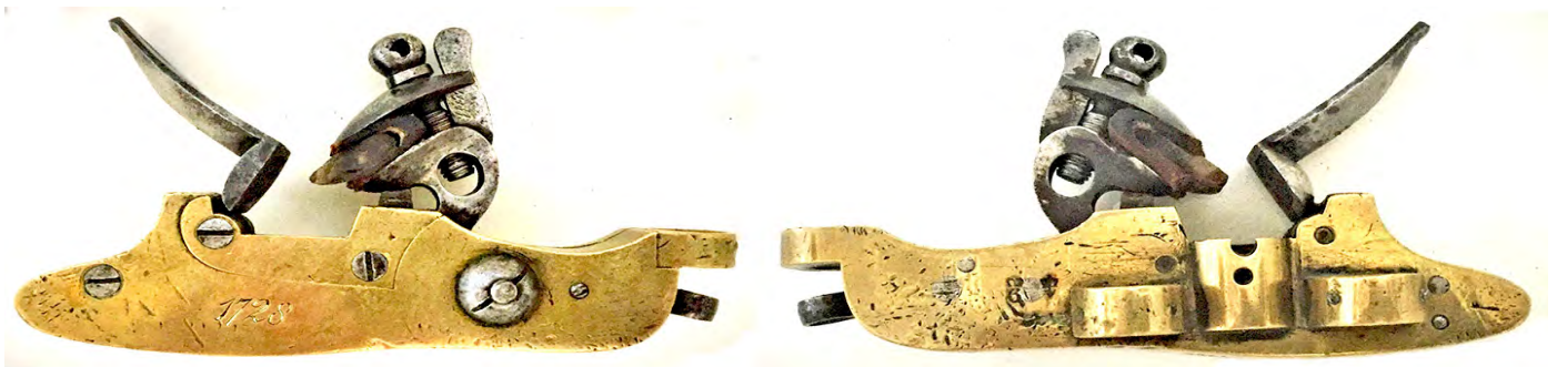
Figure 17. Maker unknown. Notice the circular forms on either side of the pan which allow vertical bolts to attach to the gun. Craig Ross collection.
