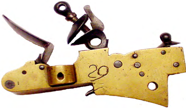
Figure 30. A French lock ca. 1800. The no. 29 indicates a particular gun this lock attached to. Notice the unusual triggering attachment. The reverse, with the maker "Brignol A Paris" stamped and the year AN13 (1806). Dick Salzer collection.
