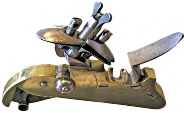
Figure 23. One of the problems with flintlock cannon ignitors was the difficulty of replacing worn out flints during the heat of battle. In 1817 Howard Douglas designed a double-headed version to remedy that concern. 5 It is doubtful that many were made because today they remain a rarity among rarities. Specimen from Rijksmuseum, Amsterdam.
