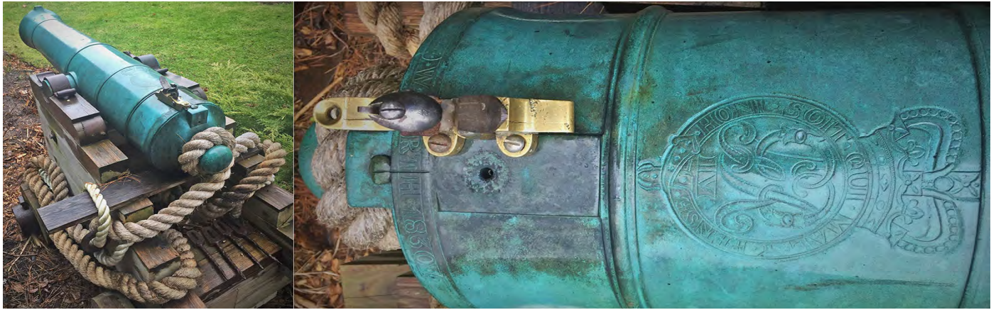
Figures 18. An 1830 bronze cannon by North, with a lock attached by vertical screws. Although it is not apparent exactly how fire from the lock is reliably channeled to the chamber, in each case there is a hole in the side or bottom of the flash pan that aligns with the channel to that chamber. Ignition was achieved by possibly using a primer charge in a quill or tin tube. Tin tube primers were unpopular with seamen of the day, who worked barefoot and often cut up their feet on discarded tin tubes strewn around the deck. 4 Without in situ examples to view, we are left to our imaginations as to exactly how it was managed in each case. The cut-a-way views in Figures 4 and 5 are typical of the principle. Craig Ross collection.
