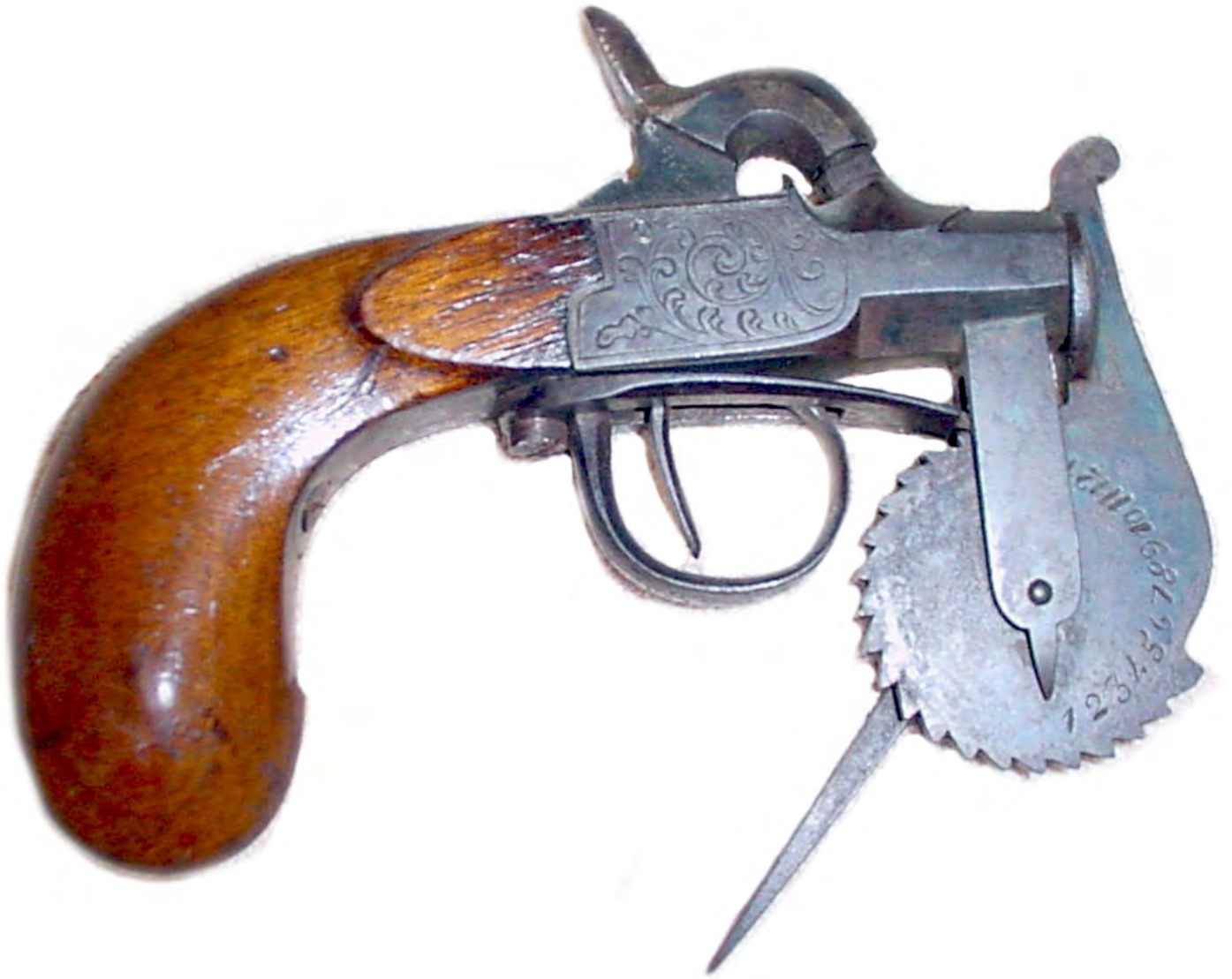
Figure 21. A simple French or English percussion tester. Accidentally buying this at a local auction it is what started me collecting powder testers.
