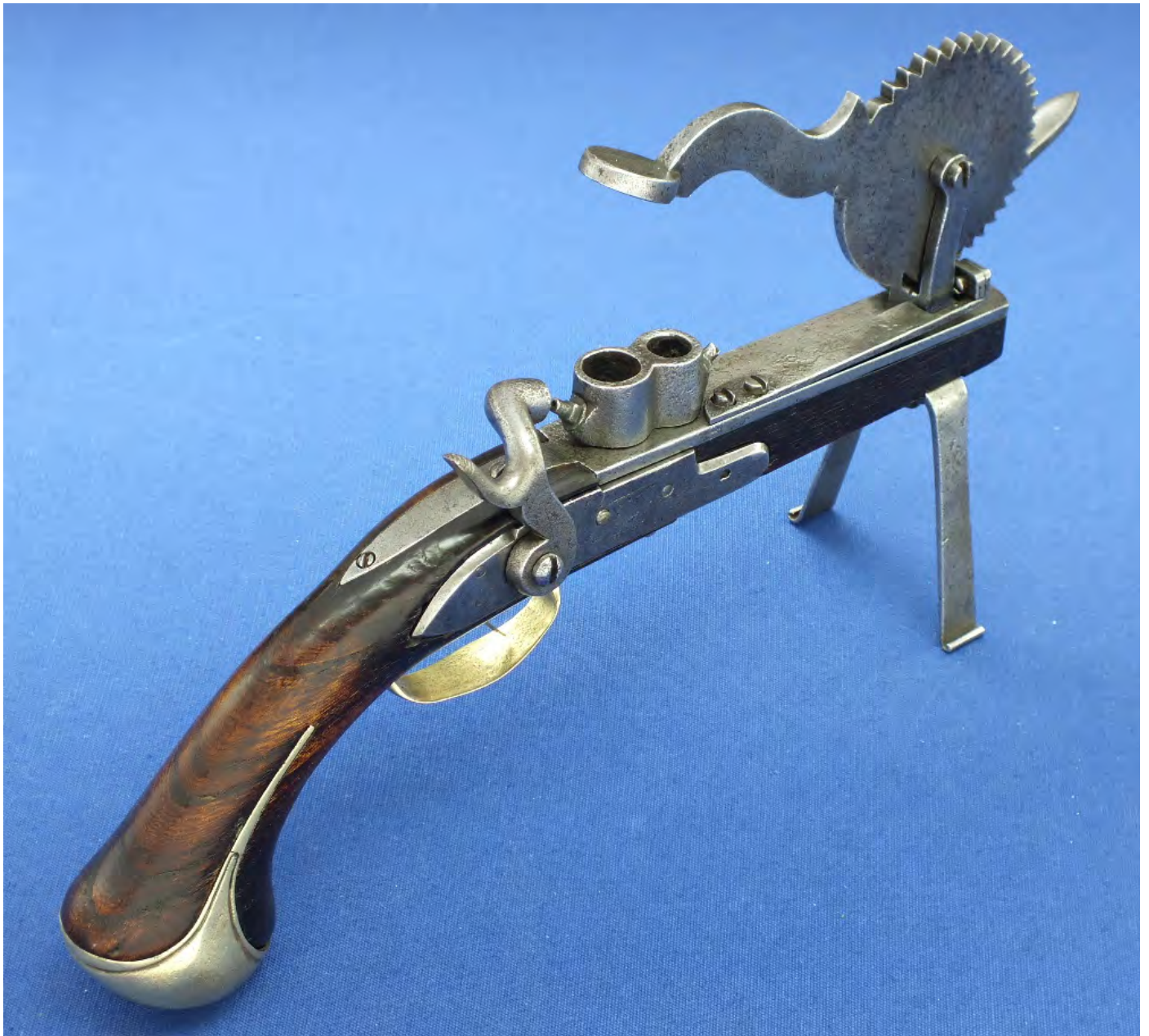
Figure 18. An unusual percussion tester from Holland. This one has two different powder chambers that can be rotated to align with the activator arm, probably from about 1840.
