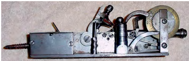
Figure 10. Probably one of the most complex devices dreamed up by an ancient inventor, this combination tinder lighter/ powder test has a gun barrel attached for good measure. It probably dates from the early 1700's.
