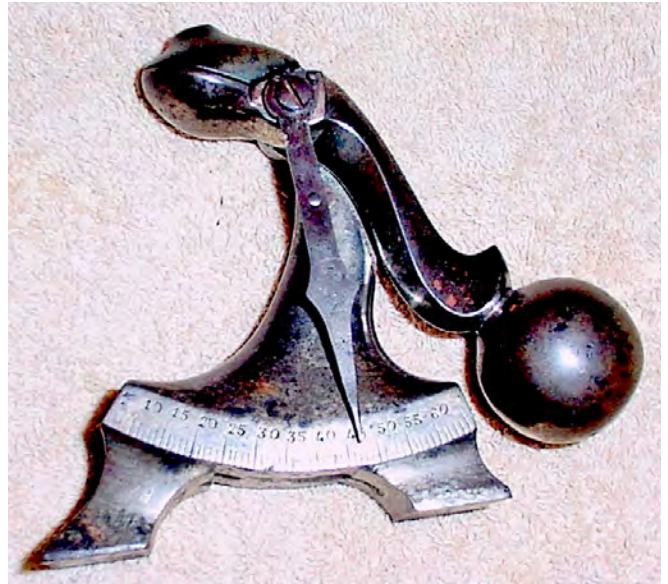
Figure 8. An early French tester, firing a tiny quantity of powder by touch-hole causes the weight to swing and the pointer to register the travel.
