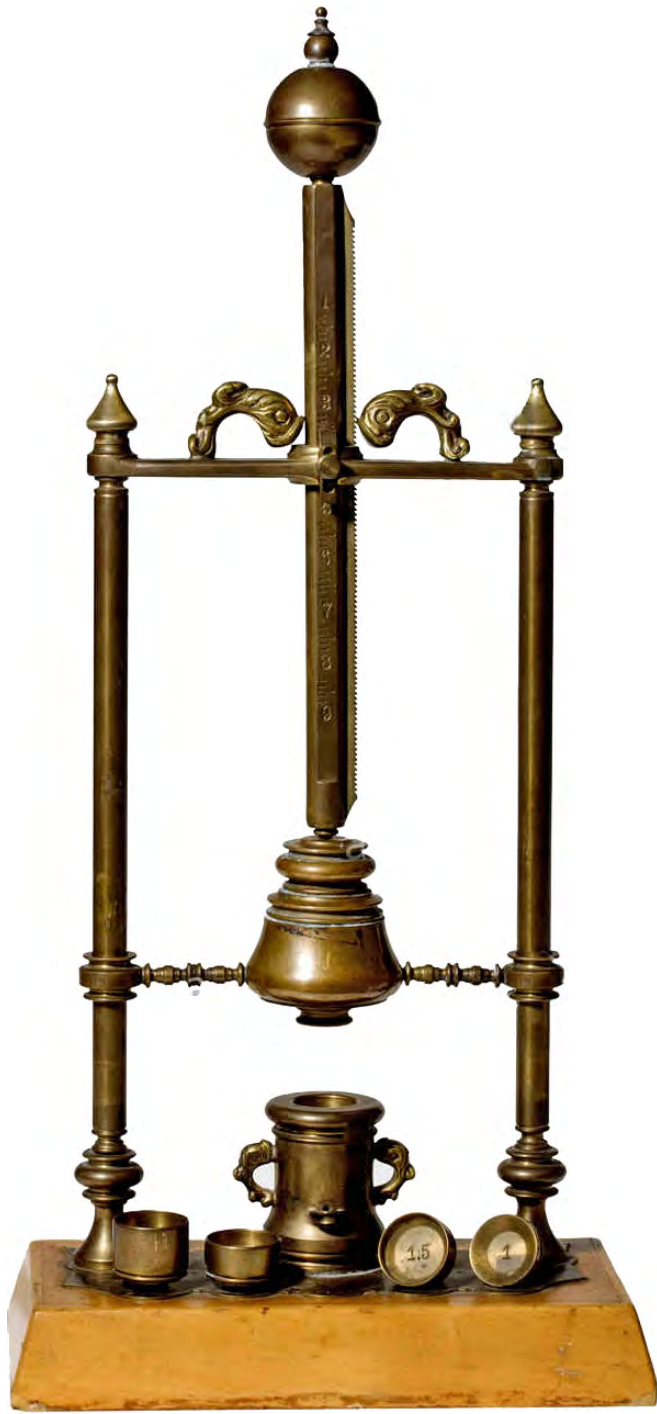
Figure 5. This elaborate laboratory tester fired weights of various sizes, vertically, to measure the height achieved. Probably dates from the mid-1850's.
