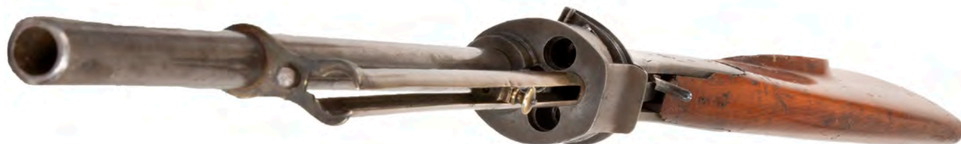
Figure 10. Underside view of the Lindner Repeater showing a single magazine tube and piston. Lindner made provisions for two more magazine tubes in the cylinder faceplate, but he did not make provisions to support additional tubes at the muzzle end.
