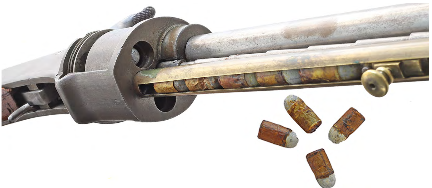
Figure 9. The loaded Lindner repeater with cartridges in the magazine tube feeding the rotating cylinder. Note the empty cylinder chamber is ready to accept the next cartridge to be fed from the tubular magazine. As no original Lindner cartridges are thought to exist, these .48 caliber x 1.00 inch-long reproductions were made to demonstrate the loading operation. Cartridges courtesy Garry James.
