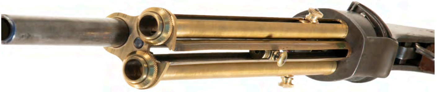
Figure 11. The author machined two magazine tubes to show Lindner's vision of increased firepower. Note that the "cloverleaf" end plate merely slips over the original end plate and the tubes are locked in with the two large, knurled nuts.
