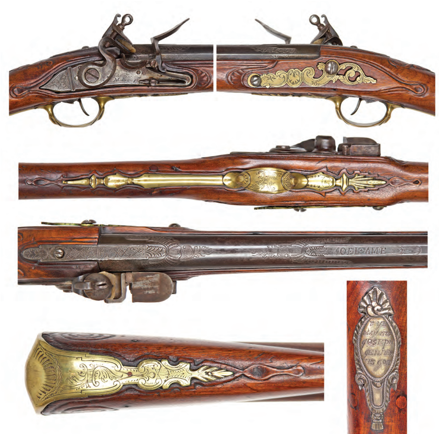
Figure 2. The French engraved lock with the American gunsmith's name, "Joel Amy", engraved under the pan has a decorative raised wood molding around it (top left, clockwise). The side plate has engraving that appears to be done in an American style rather than French. The trigger guard is French in style with the engraved design on the butt plate tang repeated on the bow of the trigger guard. The upper finial of the trigger guard is decorated with a whimsical face. The barrel tang and the butt of the barrel both have engraving that looks different from the maker's name of "JOEL+AME" engraved on the top barrel flat. The wrist plate has the owner's name in a non-professional engraving "ryE / MAY 1775 / JOSEPH JENNESS / HIS GON". The engraved tang of the butt plate has an elongated spear point form in a raised outline of wood on the stock.
