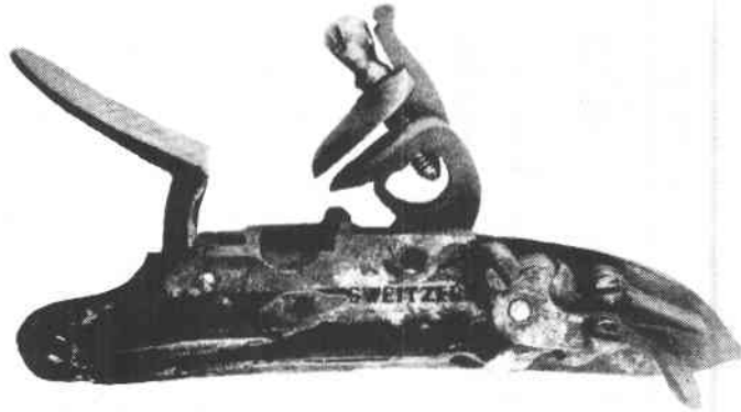
PLATE III — Inside view of the lock from a musket by an unknown maker (see "a" on Plate I). Little is known about SWEITZER'S activities beyond the fact that he was a lock maker.
