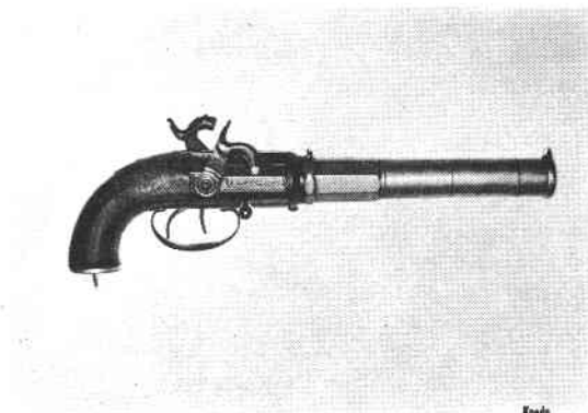
Harrington Multi-shot Pistol, seven barrel group, one nipple, all fire at once. Chamber block removes for loading.
