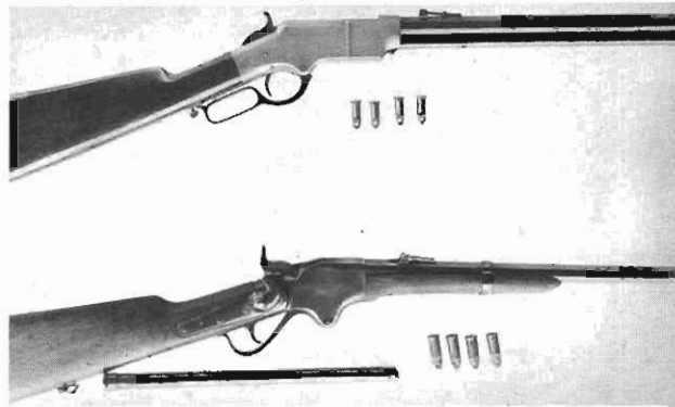
TWO OF THE FIRST REPEATING RIFLES TO BECOME POPULAR IN THE WEST; THE HENRY RIFLE, TOP, FEEDS ITS CARTRIDGES BACK TO THE RECEIVER THROUGH A MAGAZINE UNDER THE BARREL, WHILE THE SPENCER RIFLE, BOTTOM, FEEDS ITS CARTRIDGES FORWARD THROUGH A MAGAZINE INSERTED INTO THE BUTT-STOCK.
