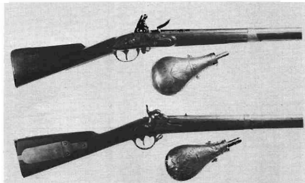
THE U.S. FLINTLOCK MUSKET (TOP) IS TYPE USED BY SAILORS OF THE PACIFIC SQUADRON IN THE MEXICAN WAR. BELOW IT, THE POPULAR MODEL 1841 CALIBER .54 "MISSISSIPPI" RIFLE.
