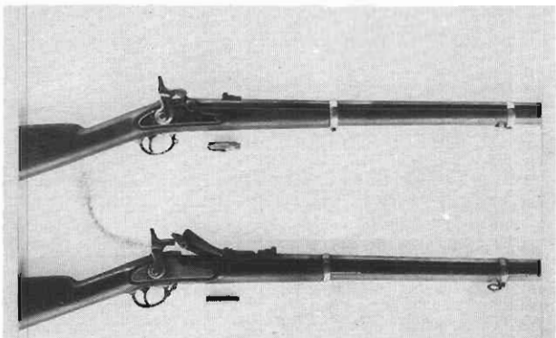
THE FIRST SPRINGFIELD BREECH-LOADING RIFLES TO GAIN PROMINENCE IN THE WEST WERE CONVERTED FROM CIVIL WAR RIFLED MUSKETS (TOP) BY A HINGED OR "TRAP-DOOR" BREECH.
