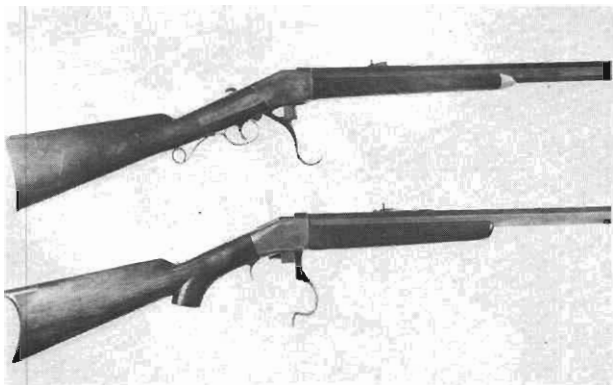
JOHN BROWNING'S RARE MODEL 1878 SINGLE SHOT RIFLE (TOP). NOTE THE LEVER PULLS BACK TOWARD THE SHOOTER RATHER THAN FORWARD AS ON THE STANDARD 1879 MODEL BELOW IT.
