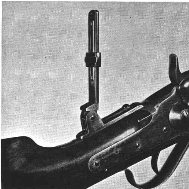
Sharps tang sight were purchased by the armory and then modified.
