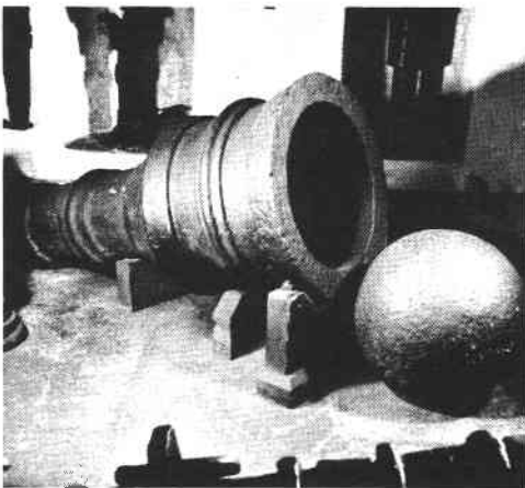
14th - 15th century Italian bombard, in cast iron, consisting of two parts: bell-shaped barrel, and movable chamber. 520 mm. bore, 1430 mm length, 1085 kilos weight. In front: a spherical stone ball for 600 mm bore bombard.
