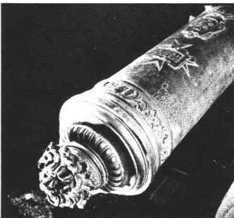
17th century Tuscan demi-cannon, modern, 130 mm. bore, 3100 mm. length, 1532 kilos weight. Cast in Florence, 1633 by Cosimo Cenni.
