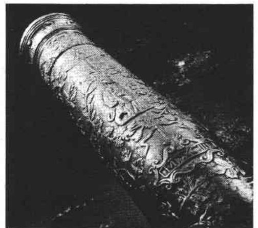
Venetian rampart cannon (modern culverin) of the 16th century. 132 mm bore, 4200 mm length, 2474 kilos weight. Cast in Venice, 1594, by Emilio Alberghetti.
