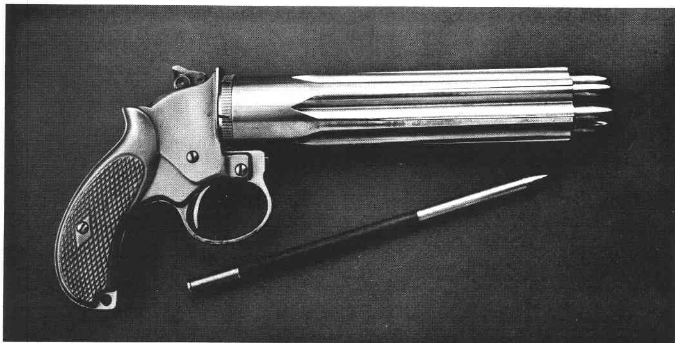
Fred Stevens underwater pistol 6 shot, stainless steel, .38 cal. dart shooting pistol. Currently in experimental production.
