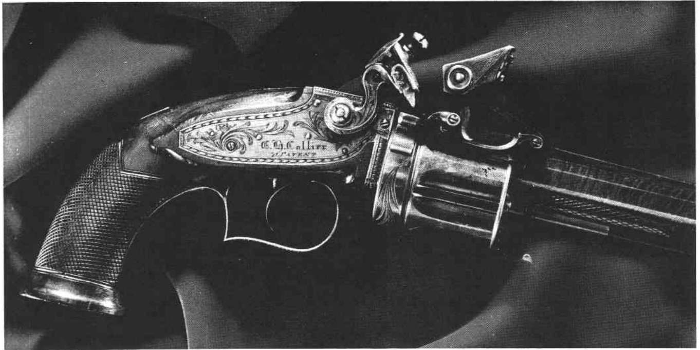
Elisha Collier's revolver. Flintlock with primer magazine made c. 1820. Frizzen engraved "E. H. Collier/71 Patent." loa. 13-7/8", bbl 6-7/16, 5 shots, cal. .46". Wadsworth Atheneum, Hartford, Conn.
