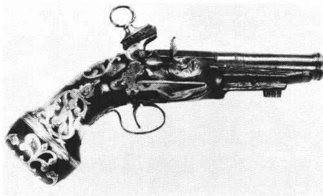
Figure 19 Eighteenth Century Type IV with iron mounts. Putto in garland on grip. Bridles do not match. Crescent cock neck with wasp-waisted plate. Mouldings along barrel and ram rod mortises. Madrid, Museo del Ejercito.
