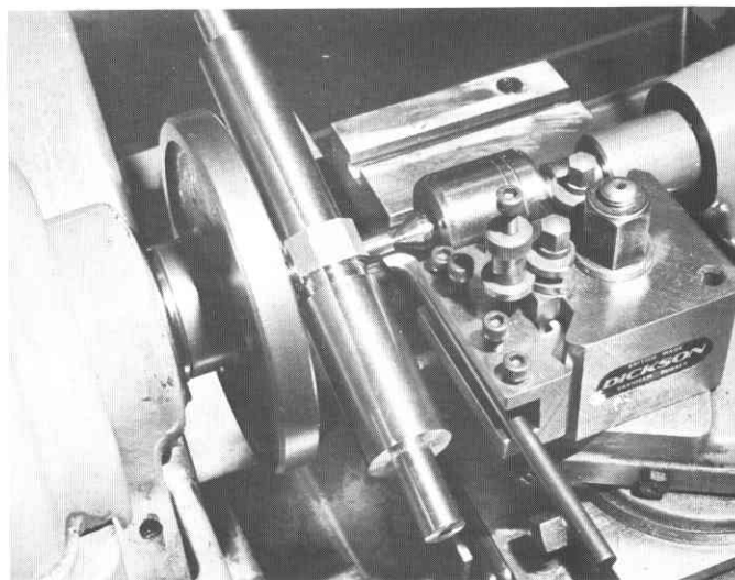
Figure 6 Lathe operations on the barrel
