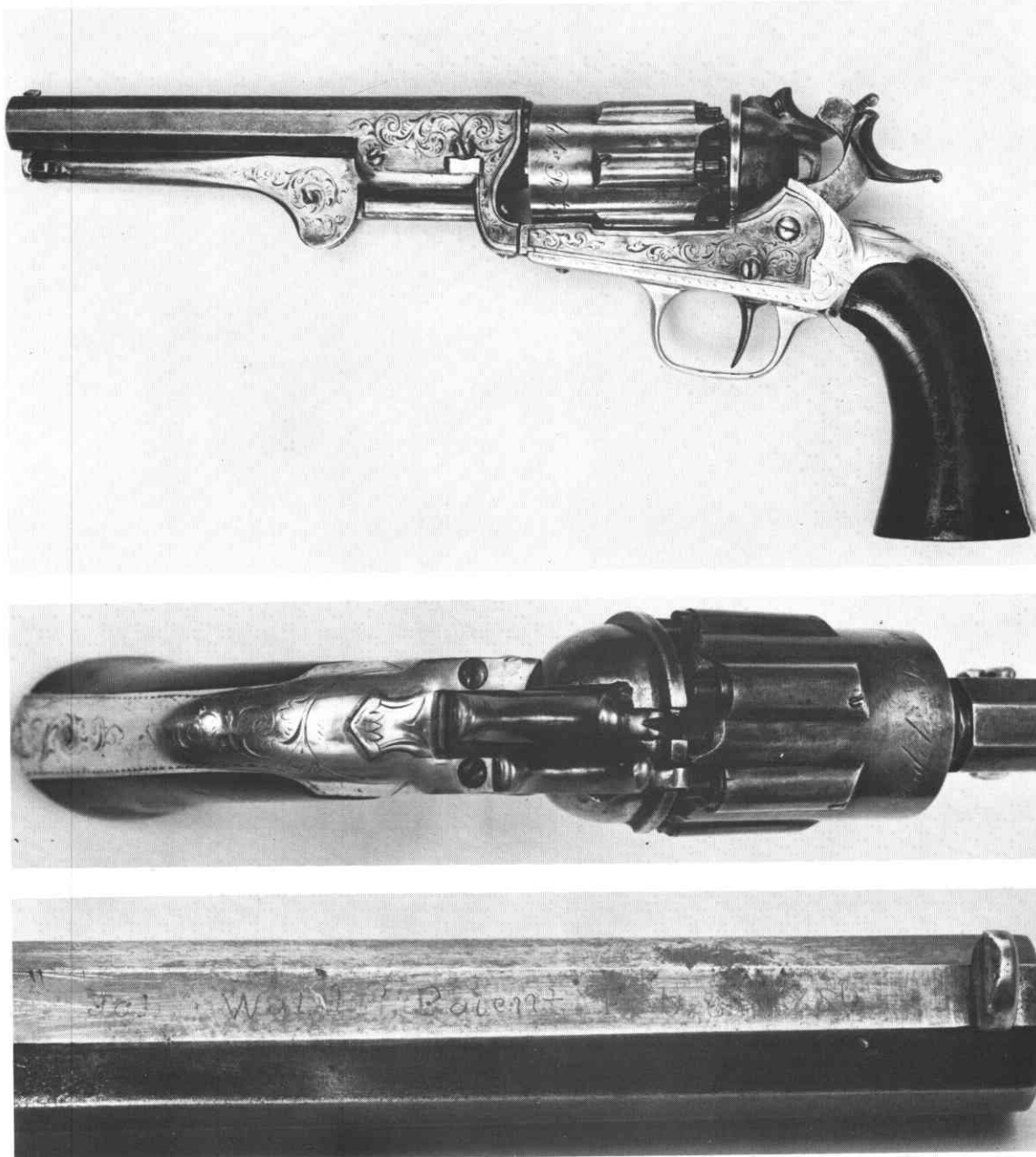
Figure 5, 6, 7 Walch 12-shot prototype revolver. Silver triggerguard and backstrap, underside of barrel marked: "Jan Walch Patent".
