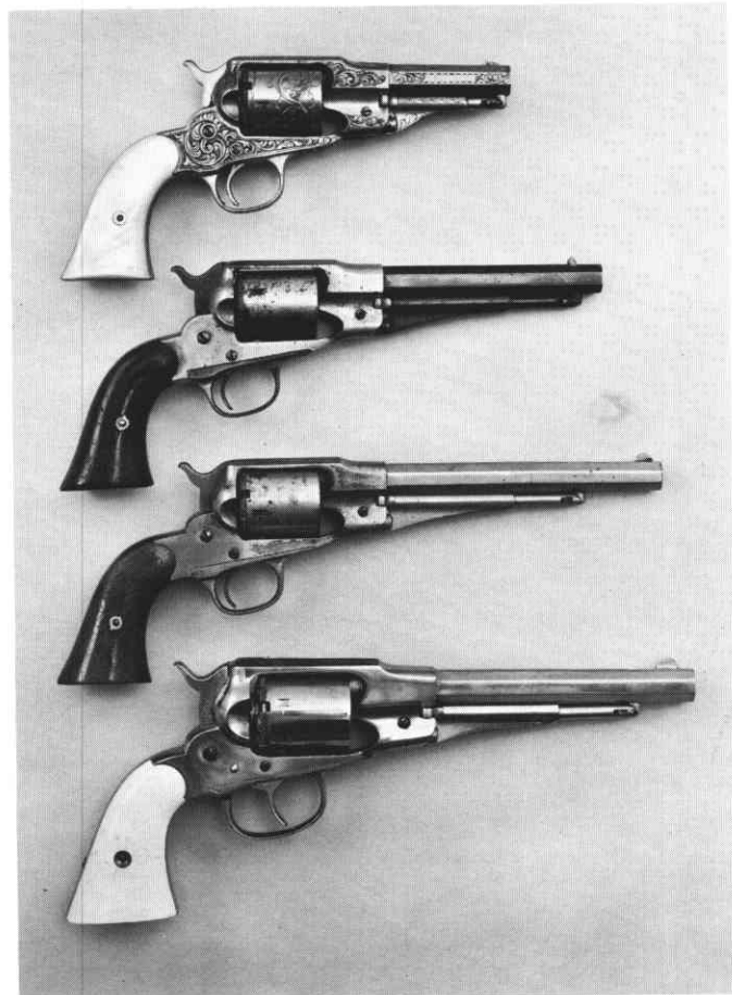
Figure 13 Belt Model conversions with back plate additions
