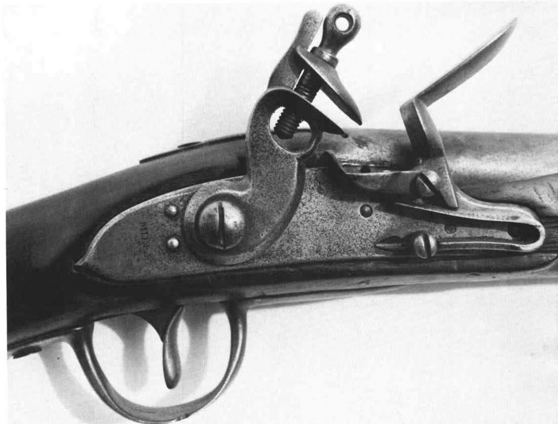
Figure 13. Miles musket showing the pan and frizzen similar to the McCormick musket in Figure 10.
