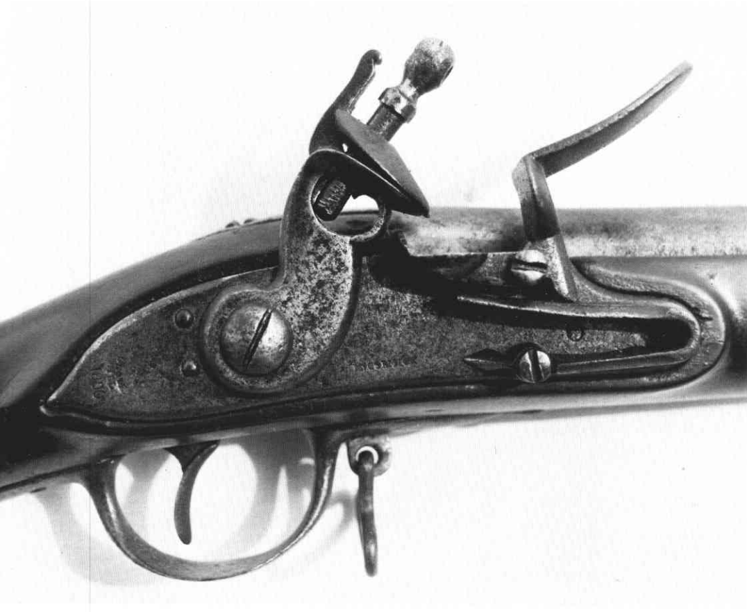
Figure 10. McCormick musket lock, showing the round pan and the frizzen with a straight toe.
