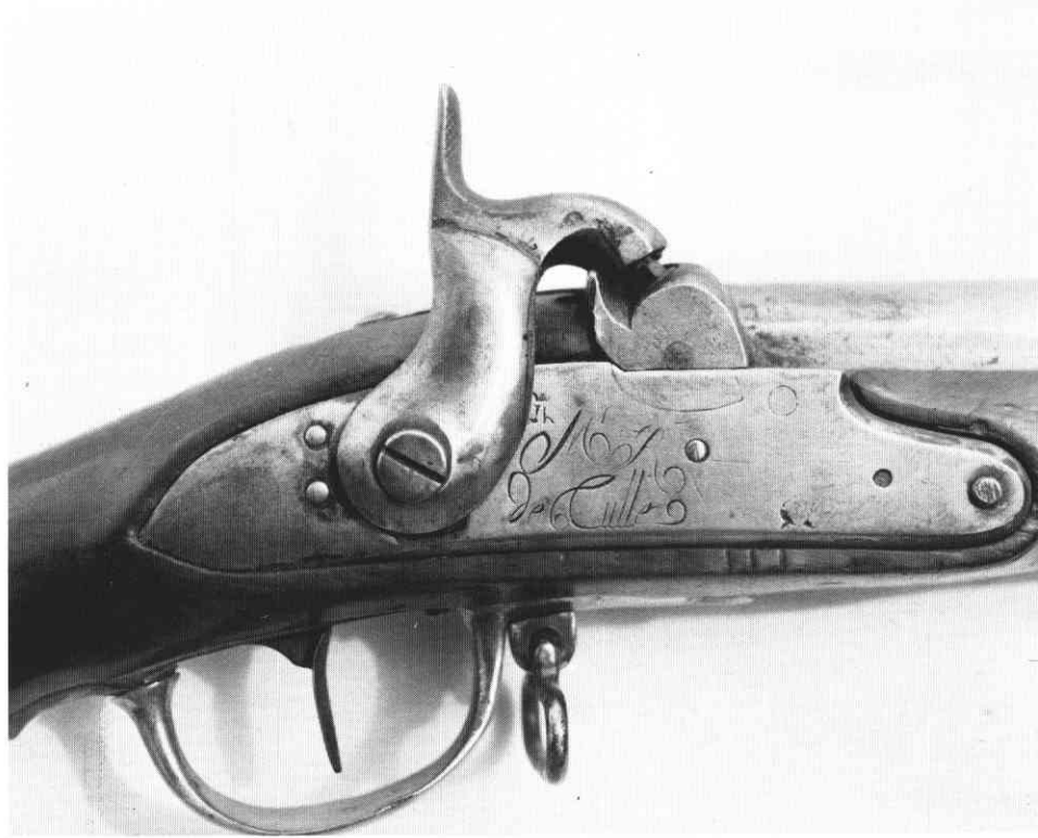
Figure 4. Close-up of converted French musket Lockplate.
