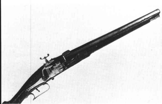
Portuguese flintlock pistol of the so called "horse neck" type, made about 1610. Note the similarity between this Portuguese pistol and many of the very early pistols made in Great Britain. Similar shape of muzzle, same large detachable pin which holds the trigger in place. Same type of three lock screws.
