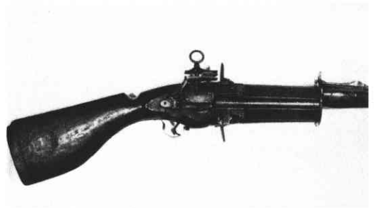
Indo-Portuguese four chambered "patilha" or so-called miquelet-lock gun made in the Goese arsenal about 1660.
