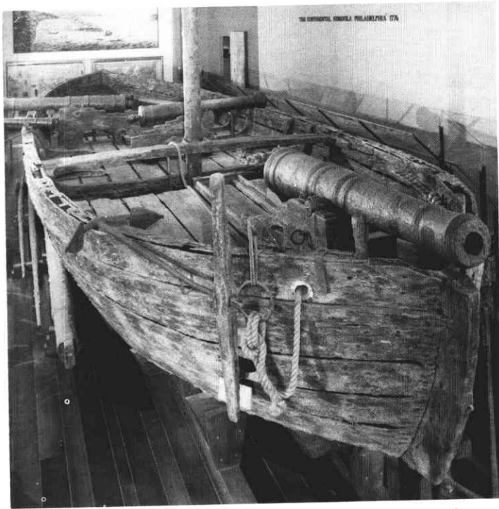
The Continental Gondola Philadelphia : Bow view showing main battery arrangement, with 12-pounder bow chaser on slide carriage.
