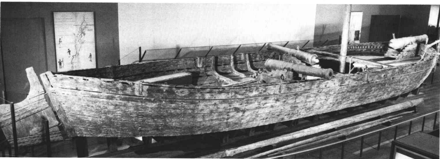
Quarter view of the Philadelphia , showing disposition of armament, including swivel brackets on gunwales. Original mainmast and spars mounted alongside.
