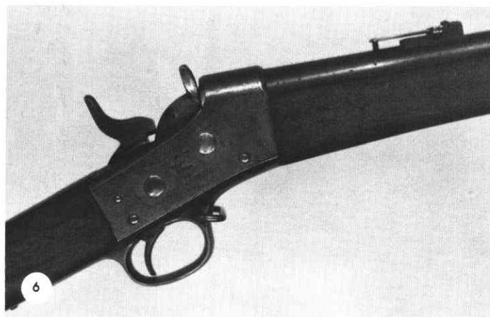
Receiver marking on both types. Traces of case hardening.
