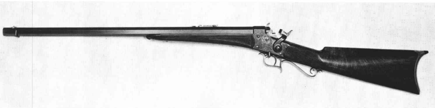
"J. Rider Patent Jan. 3, 1865". Patent no. 45,797. Engraved. Exterior left hand hammer similar to silver print in Karr's book, page 53, of 1865 prototype army pistol. Two barrels: 32 and 38 rimfire.
