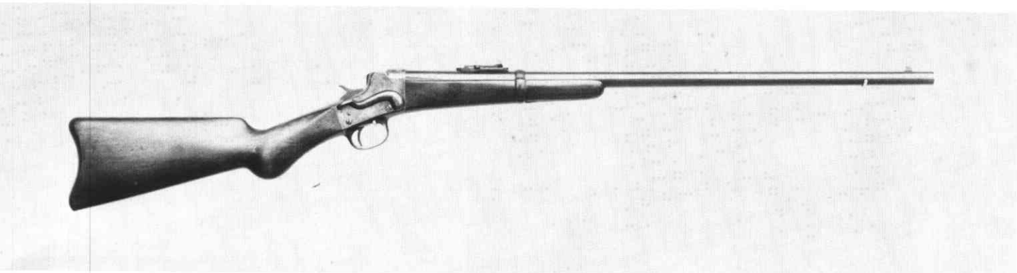
Hepburn 45-70 Experimental carbine. Extra large side lever with big thumbpiece. Barrel not drilled or tapped for second rear sight screw.
