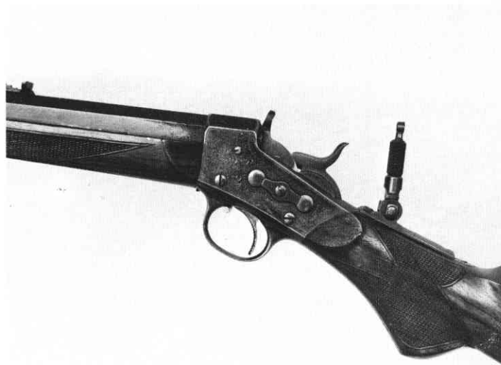
No. 2 action, engraved, pistol grip schuetzen rifle. A retirement award to a factory foreman. Rare with pistol grip.
