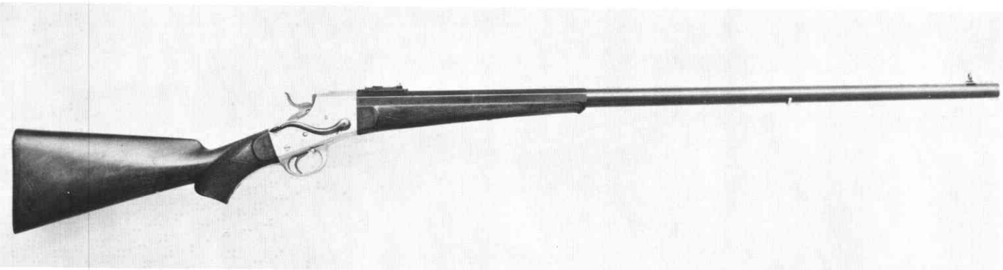
Remington plus Hepburn cross of rolling block and dropping block. Hammer rolls under dropping block — extra long side lever. Calibre .45.
