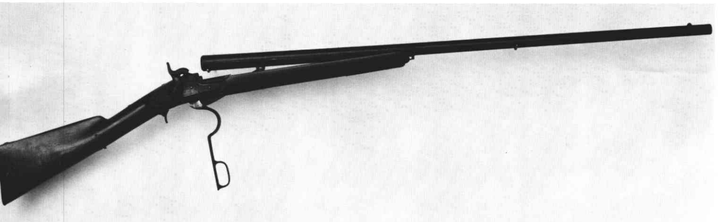
Remington percussion SS Breechloader, marked "Remington's, Herkimer, N.Y." .58 calibre. Loop lever lowers to slide barrel forward to tilt up for loading. No rear sight. O.a. 57". bbl. 40". wt. 10 lbs.
