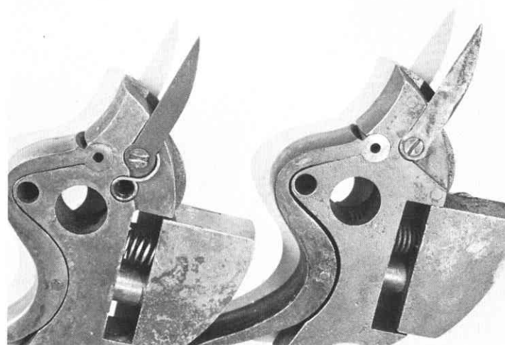
Right: Old model extractor. Left: New spring-assisted extractor.
