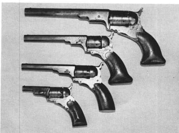
All models of Colt's rammerless Paterson pistols. From top: #5, Holster model; engraved #3, Belt model; #2, Pocket model; #1, Baby Pocket model.
