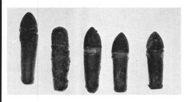
Below, left, are five skin cartridges for .36 calibre revolvers: Remington, Savage, Colt Navy (2), and Colt Pocket. With them ends this summary of standard pistol and revolver cartridges; there were paper cartridges for Sharps single shot percussion pistols, and there are other old paper and combustible cartridges of which I do not have specimens, but those shown are typical and representative of those used here and in Europe.
