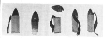
Here are some other Colt-Eley cartridges and envelopes. At the top is a further development of Adams' ball-tang: now a paper case is placed on the tang, then an iron washer riveted in place to hold the paper, which is then filled with powder and sealed. Calibres shown are .44 and .36; the uncased cartridge is a remnant of a glued-on-bullet skin cartridge, of which more in a moment.
