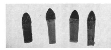
The smallest of the nitrated paper cartridges were for the .31 and .28 calibre pocket pistols. These are representative samples. The band at the bullet of the .28 calibre is a bit of scotch tape someone put there.
