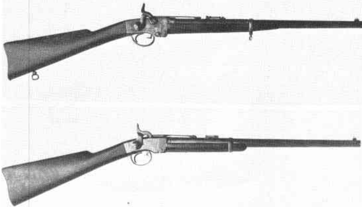
PLATE 10 Numerous features of the extremely early percussion Smith carbine shown above were changed as production began, such as the buttstock and forearm, the length and contour of the frame, the bolster and hammer, and the trigger guard. The swivels, common to early production Smiths, were eliminated in favor of a bar and ring on the reverse side of the receiver. The second specimen shown was originally made in .50 calibre rimfire after a short series of experimental percussion-to-cartridge conversions.
