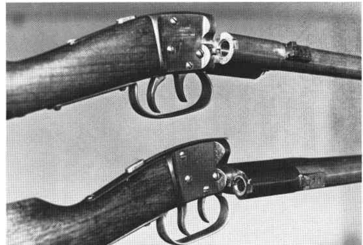
PLATE 21 The application of pressure to the finger release on the see-saw atop the receiver allows the barrel to unlock and drop to the right exposing the chamber for loading. This swinging motion at the same time activates a tiny extractor, visible in both carbines riding out over the face of the frame.
