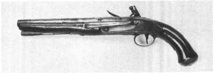
Reverse of the 1812 U.S. Navy J. Henry pistol showing the attachment of the belt hook by the rear lock plate screw.
