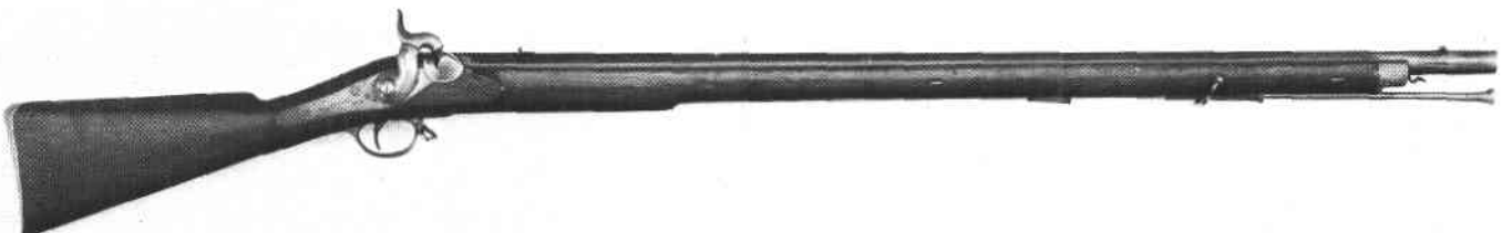
This musket was the only new made percussion musket submitted in the British trials of 1836. Short comings were found in each of the altered muskets and so in 1838 a limited quantity of Lovell's cap muskets were produced and these became known as the Pattern 1838.
