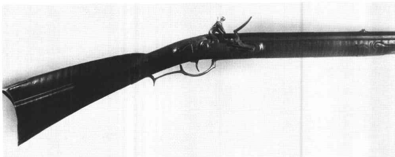
The first rifle in this review is probably the earliest. Its single most interesting feature is its sliding patchbox cover which is used instead of the customary hinged-lid type. The severity of design and lack of decoration sets it apart from many other later rifles.
