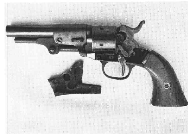
Experimental cup-fire revolver from 2nd Model percussion parts.
