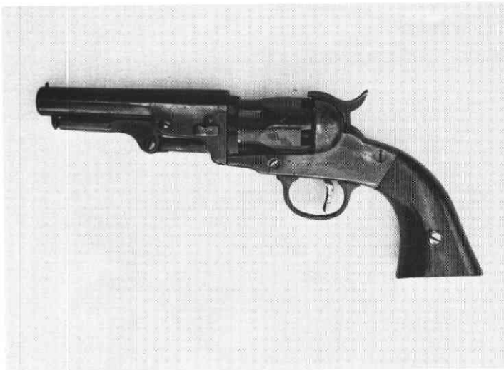
Marked only "cast Steel"; made from left-over 2nd and 3rd Model parts.
