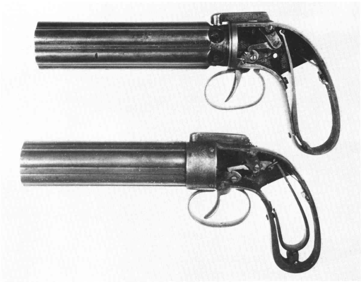
Serial 11, bottom, comparing the 1845 raised spring tension screw with the lower 1837 screw above.
