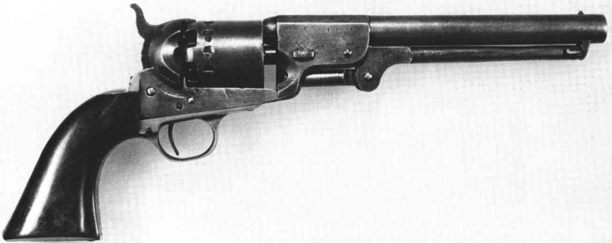
RIGDON & ANSLEY #2091: Note 12 cylinder stops and rear trigger guard screw breaking out side of trigger guard.
