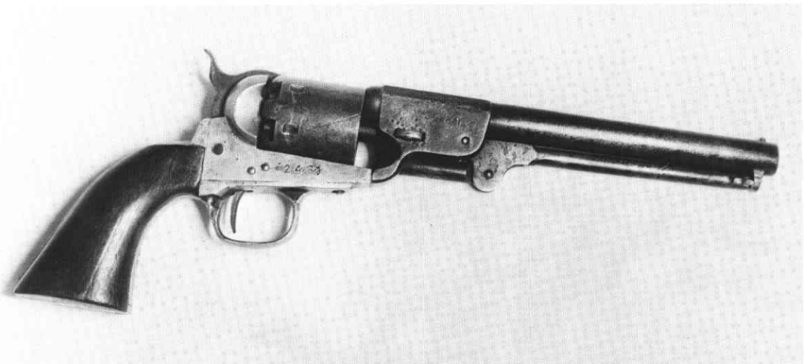
Fake GRISWOLD & GUNNISON: Note wrong dies for serial number, wrong shape to trigger guard, and fake twist marks on the cylinder run in wrong direction.
