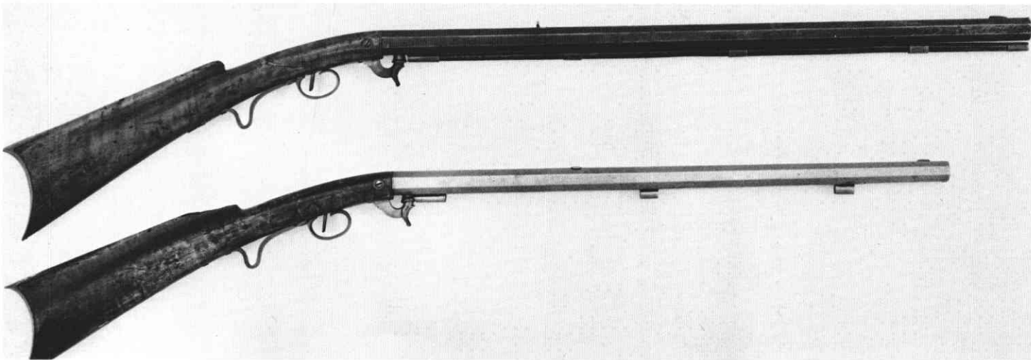
Underhammer rifle stamped N. KENDALL WINDSOR VT PATENT. 28 in. barrel; .42 in. cal Serial No. 504. Similar rifle inscribed SMITH'S IMPROVED PATENT STUD LOCK. Serial No. 302.
