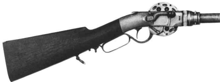
Porter's Turret rifle, patented 1851. Serial No. 660. 28 in. barrel; .50 in. cal. 14-groove rifling. Bought by the Board of Ordnance, London for trial in 1853.
