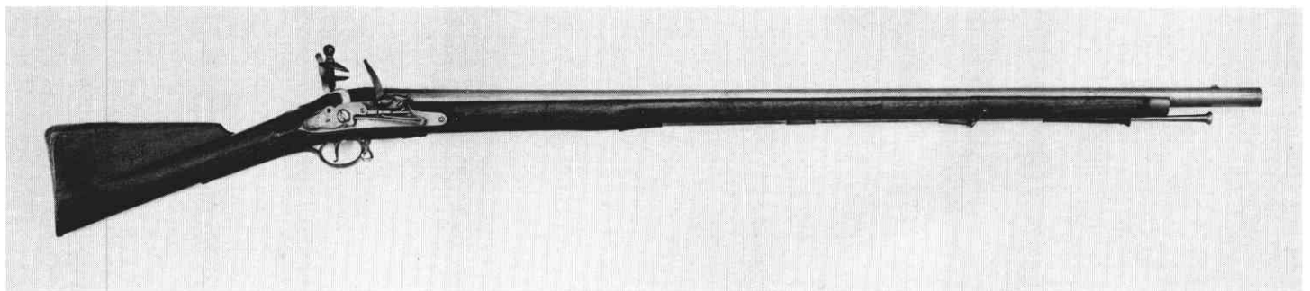
Walter Dick’s experimental flintlock, 1786; fitted to a short land pattern musket. One of three made in 1787. A single external spring acts as mainspring and frizzle spring. Dick was a Charlestown gunsmith who came to the Tower of London after the Revolution.
