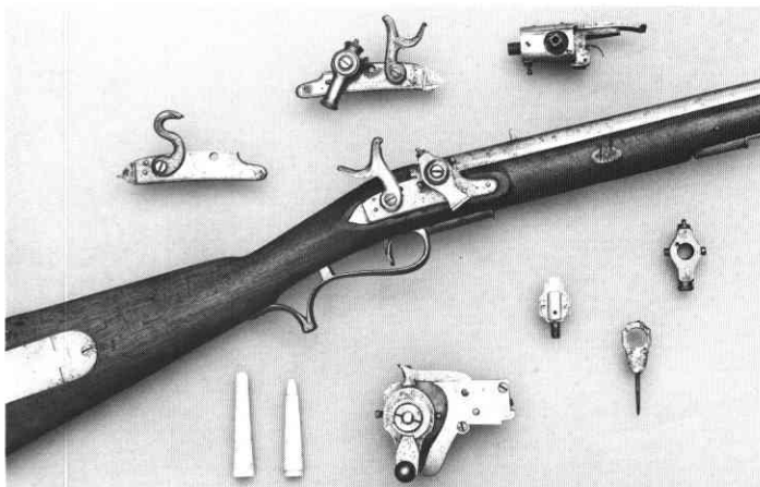
Experimental Forsyth lock mounted in a Baker cavalry carbine, ca. 1807, and other Forsyth pieces.
