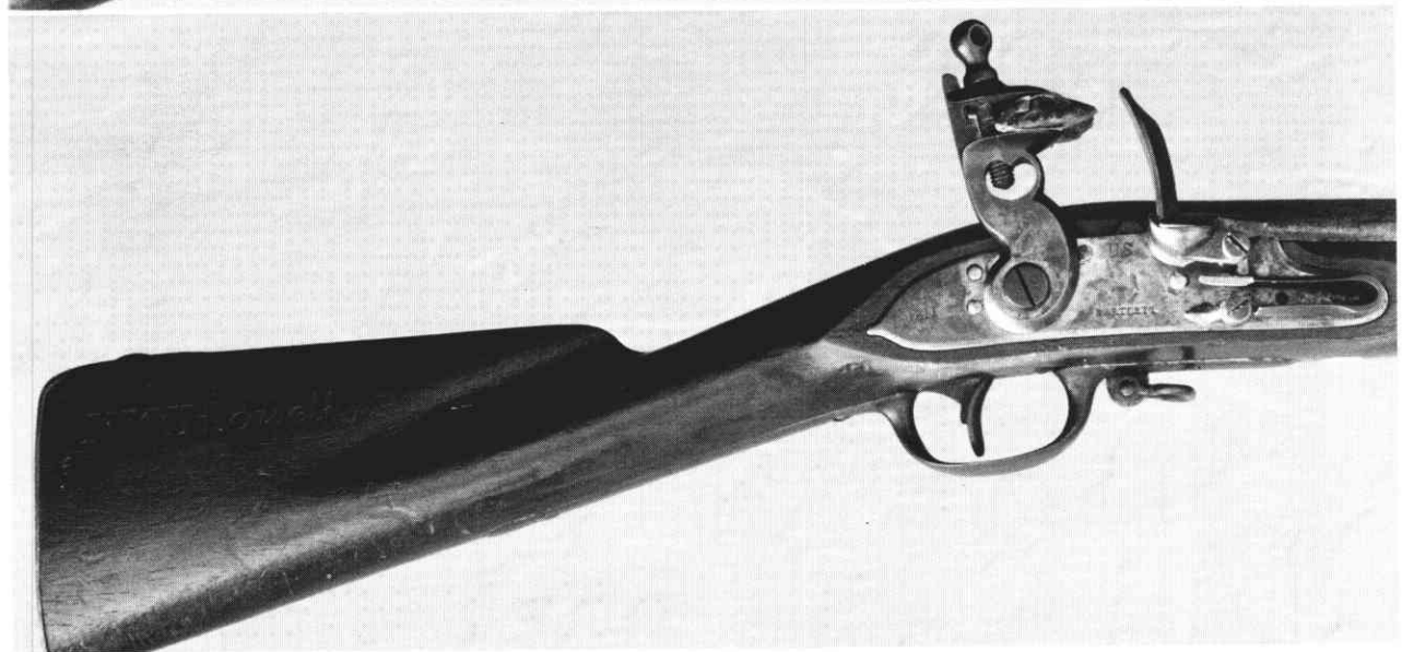
1808 Contract muskets: top - William and Hugh Shannon. Their pattern was a Harpers Ferry musket; note cock, frizzen, frizzen spring configuration, and shape of stock. Bottom - Bartlett musket patterned after Springfield; again note the similarity. The indentation in the tip of the frizzen shows well.
