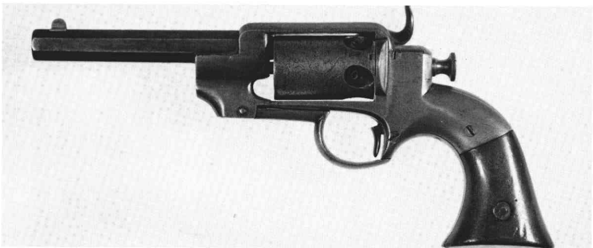
The next series we shall examine are the .28 caliber pocket models. The first model shown here has a three screw side plate. Early markings the same as the first model .36 Navy and it has the friction latch rammer. The main difference in this model is that it has the square front cylinder pin and late type cylinder. I have never seen a pocket model with an early type cylinder. Now that I have said that one will surely turn up.
