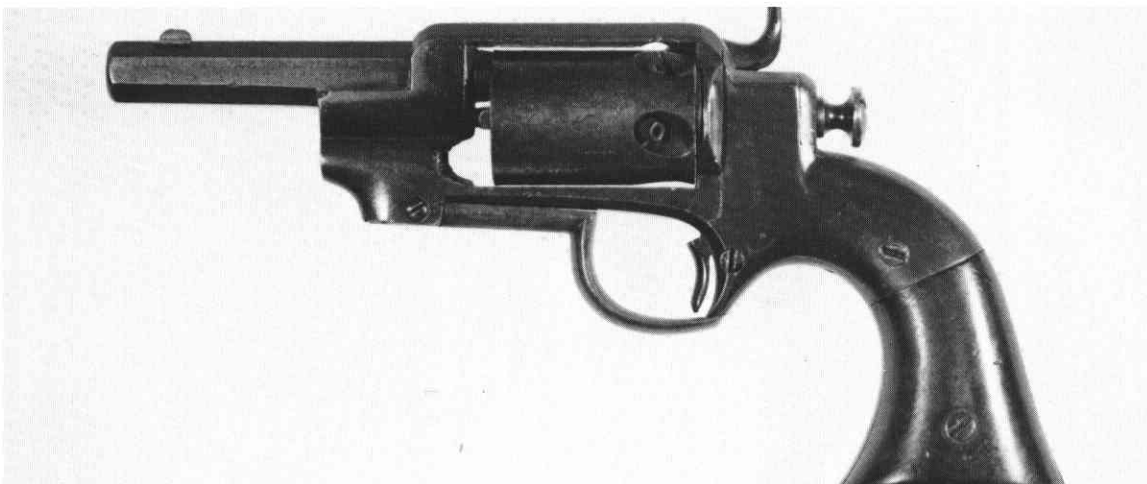
This shows the second model pocket revolver. It has a different side plate with only two screws; otherwise, it is the same as the previous piece. It has the last of the friction latches in these guns.
