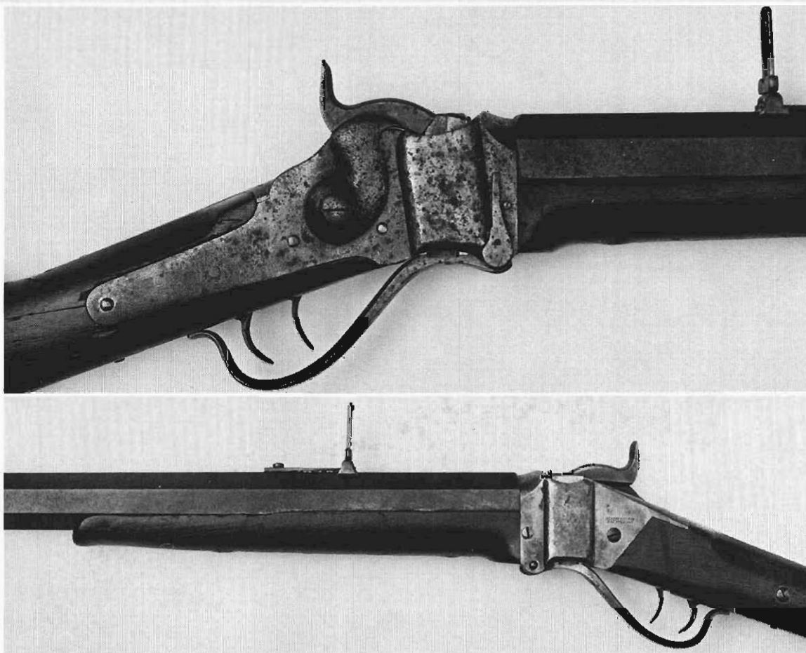
Sharps Model 1874 Sporting Octagon Rifle serial #162075, shipped to Conrad & Rath, Fort Griffin, TX, October 29, 1877, calibre 45 2/4" 30" oct. barrel, double triggers, weight 15 lb. 9 oz., cost $46.00 list. Author's collection.
