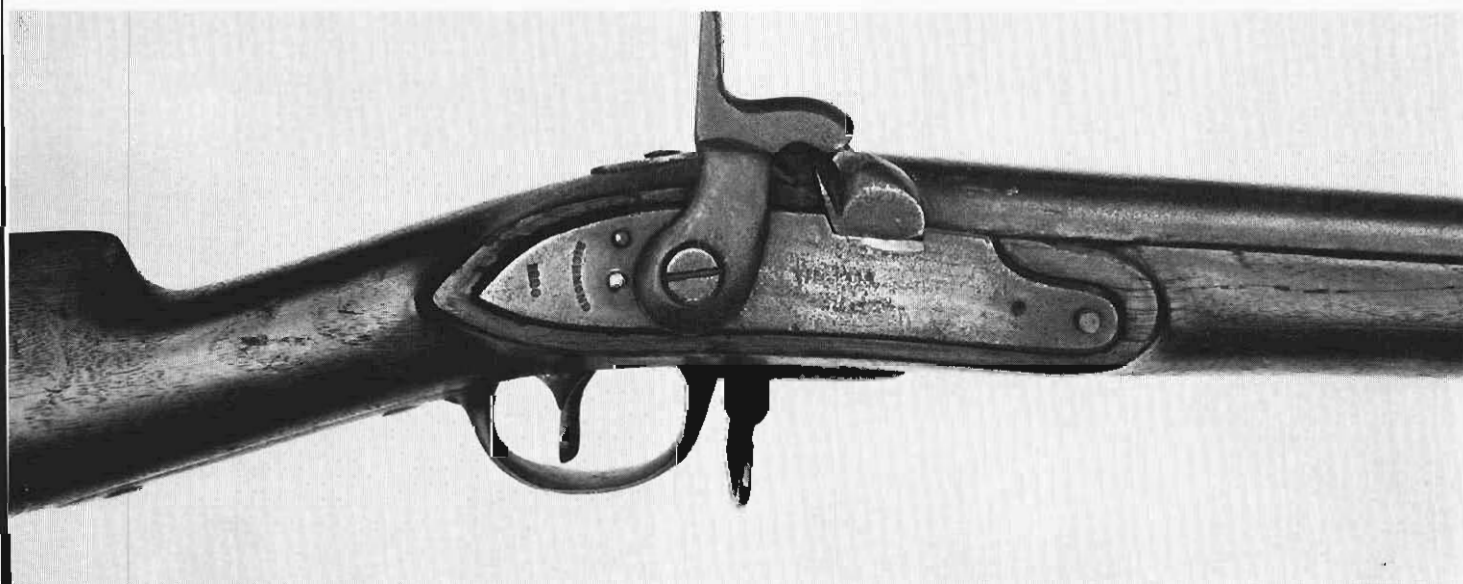
A close-up of the altered lock of the preceding musketoon. Notice the small sliver of brass from the original flash pan which has been retained at the bottom of the bolster.
