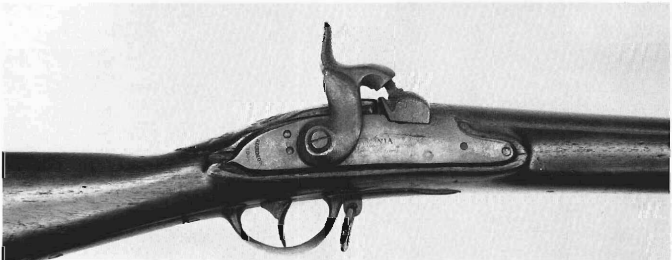
An 1804 dated Virginia Manufactory musket illustrating a S.C. Robinson alteration. The hammer has been replaced and is probably not original to this alteration. Alteration assembly/lot markings are "27" over "1".
