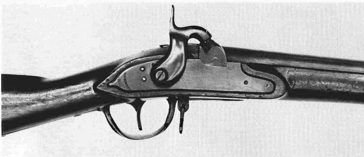
An 1803 dated Virginia Manufactory musket illustrating a Francis Perpignon alteration. Alteration assembly/lot markings are "M" and "XII."
