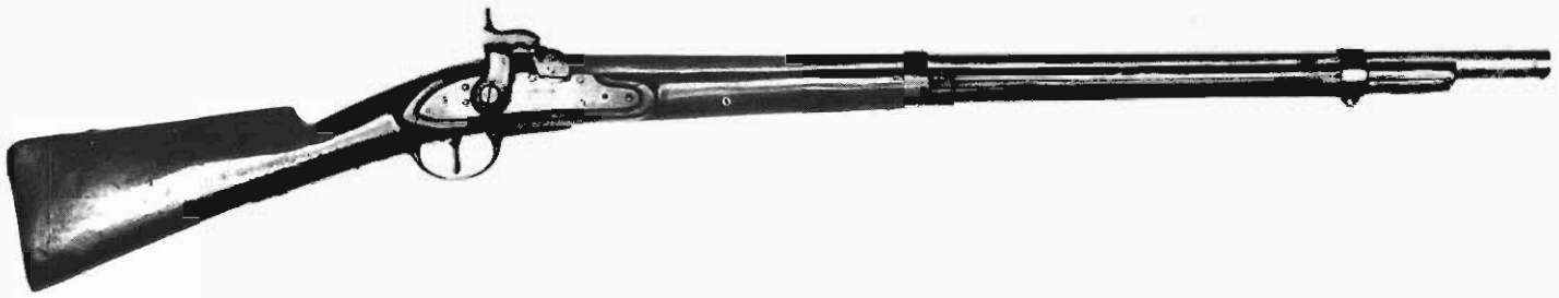
An 1818 dated Virginia Manufactory musket illustrating a S.C. Robinson alteration. This example has also been shortened, of course, but the length reduction has not been verified as Confederate at this time. Alteration assembly/lot markings are "0" and "16" over "7."
