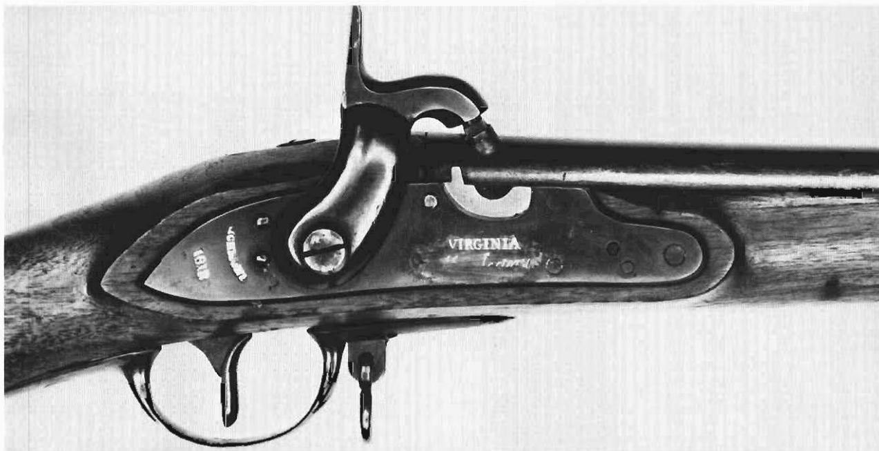
An 1818 Virginia Manufactory musket illustrating a J.B. Barrett alteration. No alteration assembly/lot marking.
