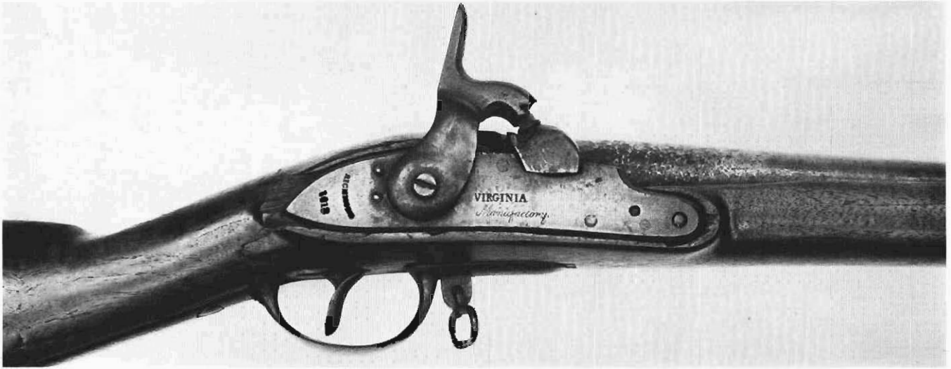
An 1818 dated Virginia Manufactory musket illustrating a typical brazed bolster alteration to percussion.
