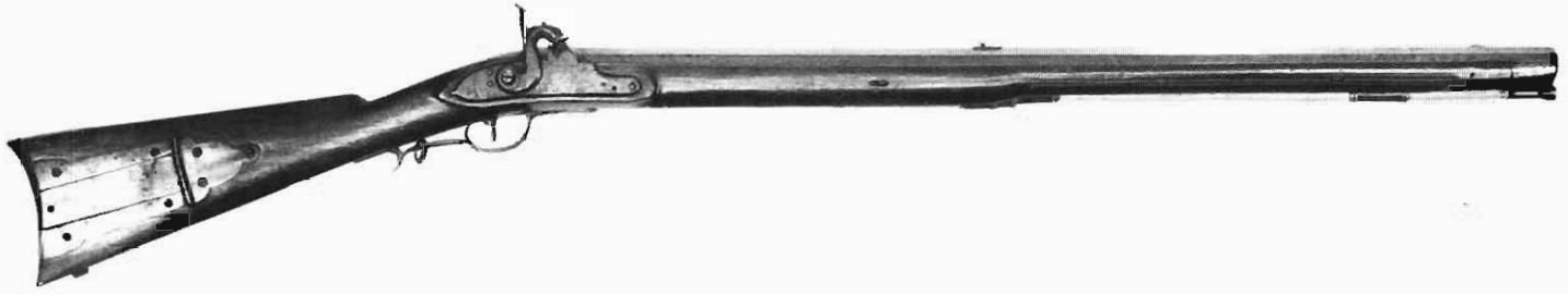
An 1821 dated Virginia Manufactory rifle illustrating a T.J. Adams alteration. This example has been shortened, probably for cavalry use. Alteration assembly/lot marking is "I.III." The hammer may be a later replacement but appears to be contemporary with the rifle.
