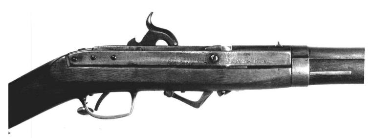
The lower carbine shows the elbow lever unlatched and thrown forward; the breechblock is still in the firing position.
