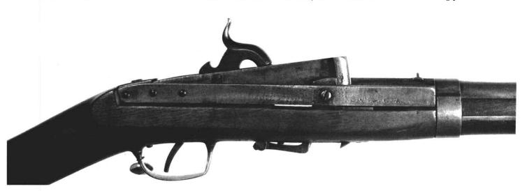
The elbow lever pushed upward and the breechblock ready for loading.
