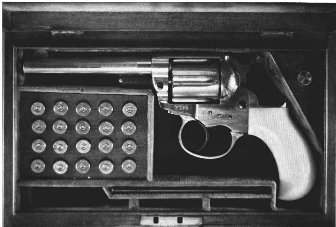
22. Serial #1031, .38 cal., 4 1/2 inch barrel without ejector, British proofs, one-piece ivory grips, shipped July 10, 1877, to Colt's London Agency and cased in original cherry box lined with red baize or felt.
