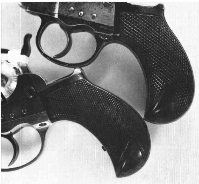
19. One-piece rosewood grips, coarsely (top) and finely (bottom) checkered; note upper revolver without the mainspring tension adjustment screw and the lower with the tension screw.
