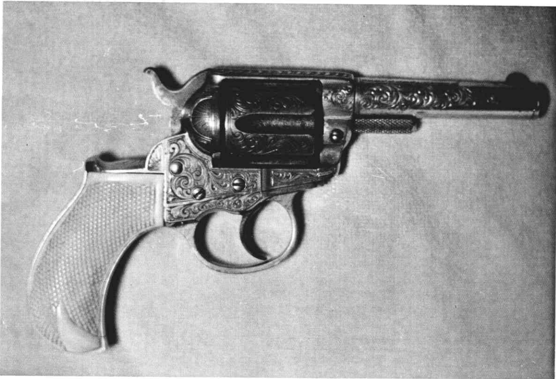
27. Serial #128, .38 cal., 3 1/2 inch barrel without ejector, nickel finish, one-piece checkered ivory grips, probably engraved by L.D. Nimschke and selected as a promotion piece; earliest known engraved Lightning.
