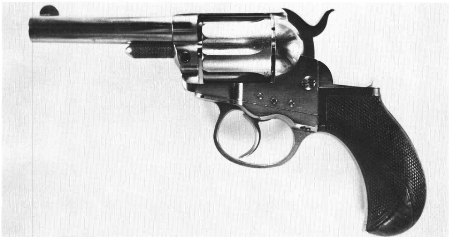
13. The "M" or Model gun, Factory prototype developed by William Mason; .38 cal., 3 9/16 inch barrel, without ejector, one-piece checkered rosewood grips, finished "in the white" (polished); "M" stamped on barrel, frame, cylinder, inside grip strap, and on hammer; "M" and "DA" stamped on cylinder pin; no patent dates, barrel address, or other markings; no checkering on hammer spur.
