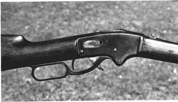
Prototype of John Marlin's first lever action rifle, which was never placed in production.
