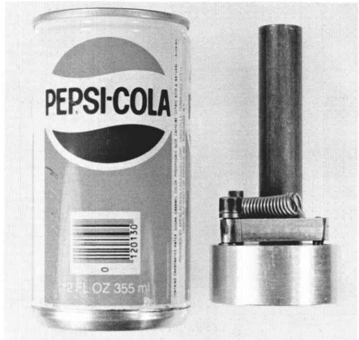
Figure 44. Pepsi Can Gun. (Can to left, mechanism to right) USA 1980. .50 percussion. Anonymous maker. Serial No. 5. RS-1.
