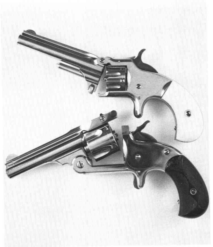
Figure 18: The Model 1 1/2 Centerfire represented a departure from tip up to top break design.
