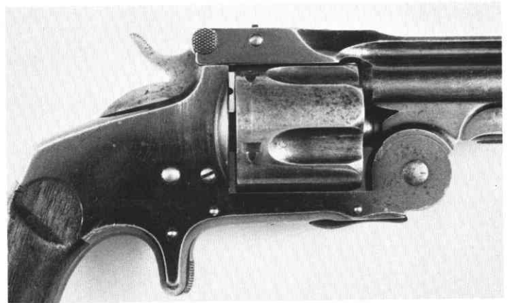
Figure 26: Detail: Showing extra screw for Aldrich 38 hammer
