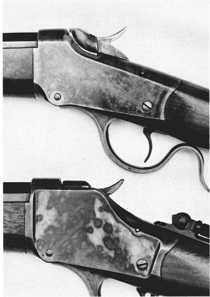
Here we see the difference between the low wall flatside (top) and the standard high wall action.
