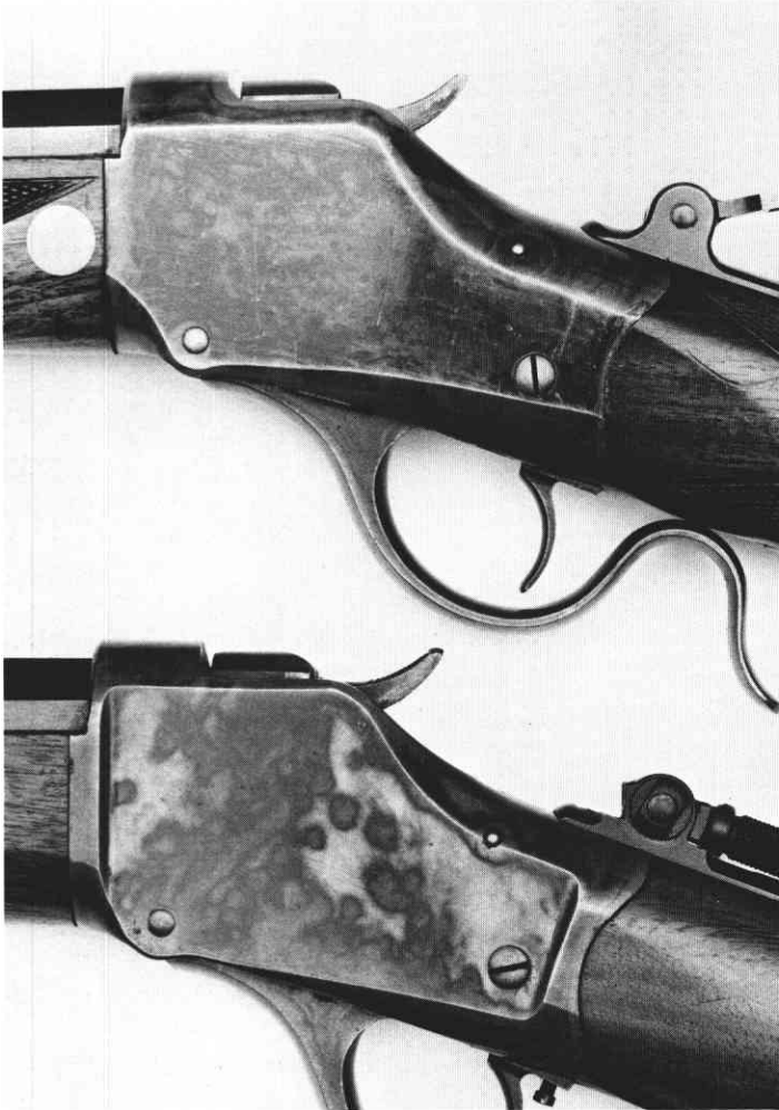
The top action is a high wall thick side or flat side. The bottom action is the later standard high wall with the flair at each end to accommodate the wood. Note the early case coloring. The switch to blue receivers was made in 1901.
