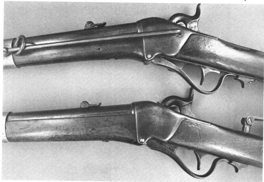
Left side of a serial no. 45, top, showing sling ring slide, compared to a civilian carbine, serial no. 1328.
