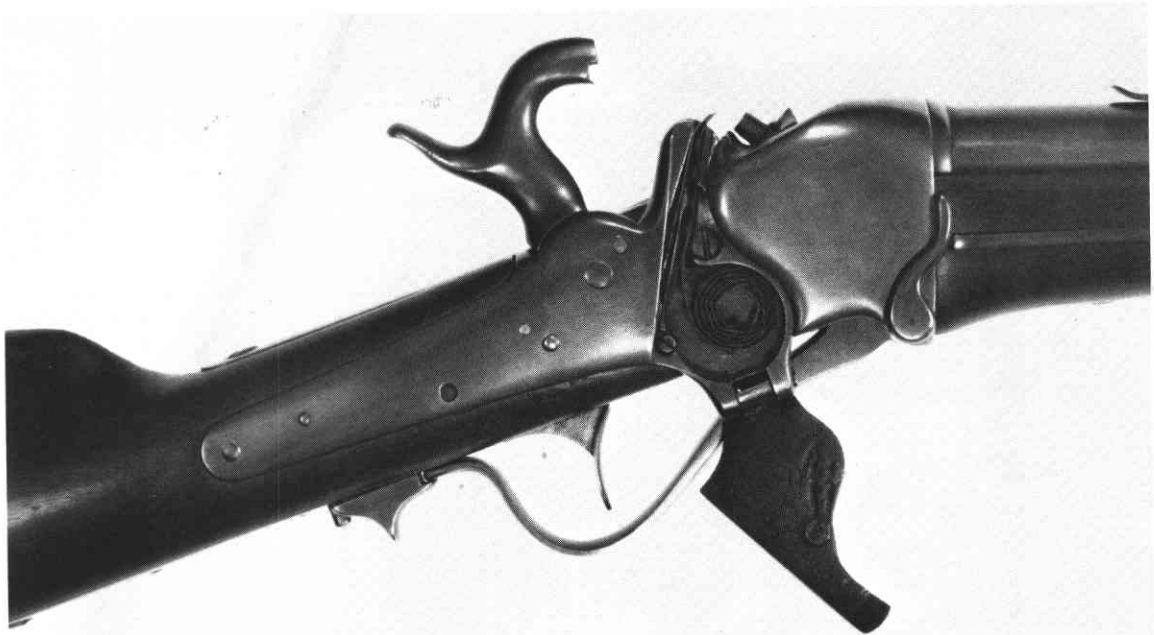
U.S. military carbine showing Maynard priming system. Note that there is no serial number on inside of Maynard priming system cover on this model.
