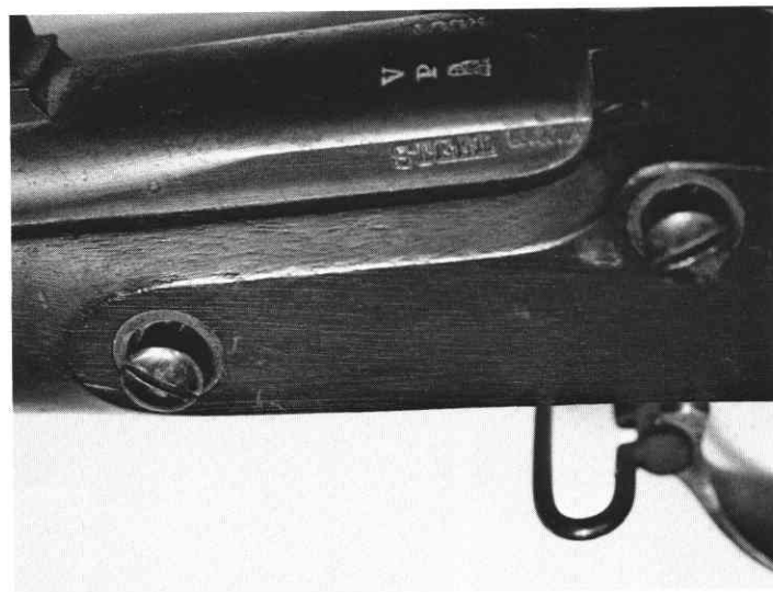
Musket lock plate screws in position for lock removal
