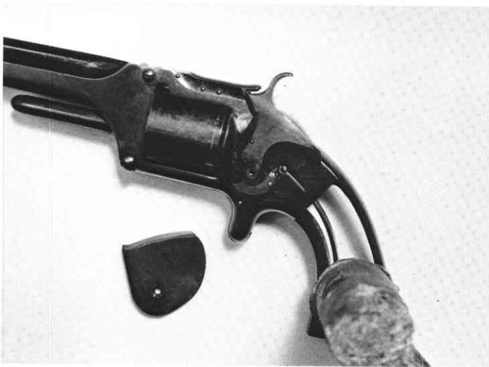
Rawhide mallet removing side plate from Smith & Wesson No. 2 Army.
