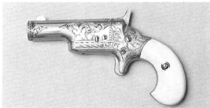
Figure 3: 3rd Model "Thuer" Deringer. Early style with high hammer, tight radiused grip strap and factory engraved.
