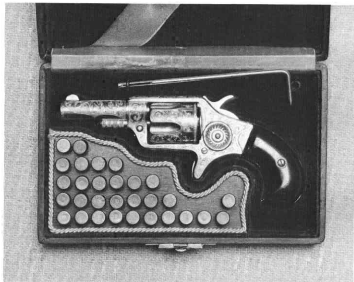
Figure 17: Factory engraved 1st Model New Line .32 caliber with locking notches on periphery of cylinder in deluxe factory casing.
