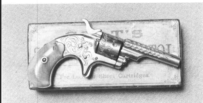
Figure 12: The last type of Open Top .22 with short barrel and low hammer profile.
