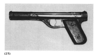
Eye pattern, but the barrel is .805 inches wide vs. .785 for the Bulls-Eye, a flattened .760 inch at the back vs. .800 inches, and 1/8 inch longer than the Bulls-Eye. The bottom, below the barrel, has a hand-cut Sharpshooter pattern trigger guard, the trigger design shown in the third patent drawing, and ca.  $1-1/2 \times 3 \times 3/8$  inch unfinished hardwood grips held by two common wood screws.
