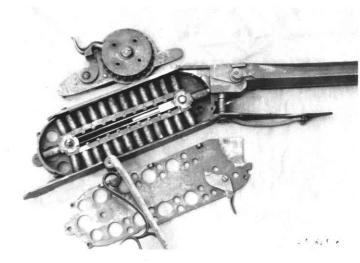
Now the ramrod has pushed a cartridge into the chamber. Note nipples on wheel above, trigger on plate below.
