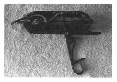
The action out of the frame: lever full down, ramrod and nipple wheel arm forward.
