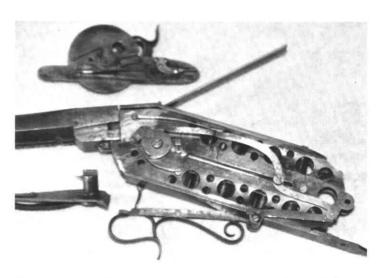
The trigger guard lever starts down, ramrod starts forward, nipple wheel arm slightly forward.
